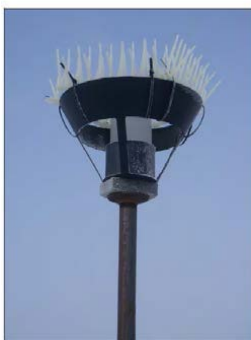
Photo 1: Dustfall collector sampling apparatus (from Rescan 2012).
