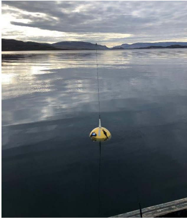
Photo 3-1 Demonstrative Photo of Drogue Deployment, Photo taken in Arctic Bay
