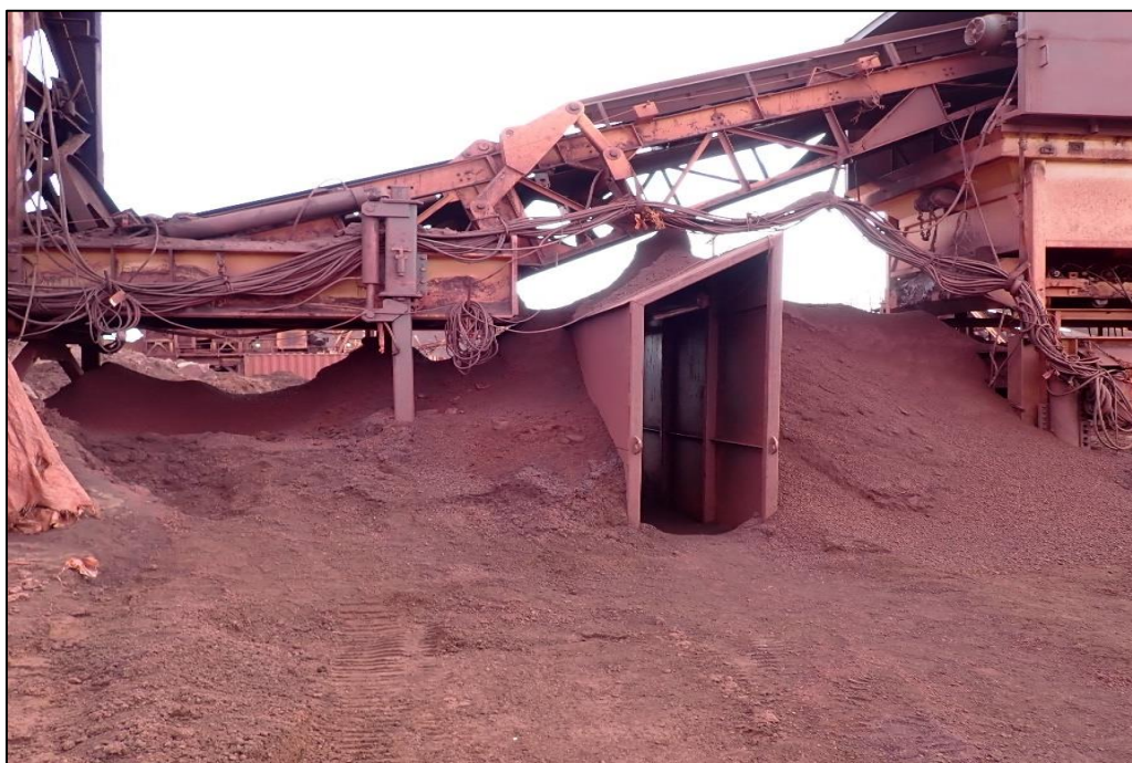
Photo 14: Iron Build-up Under Crusher Equipment at Transfer Point
