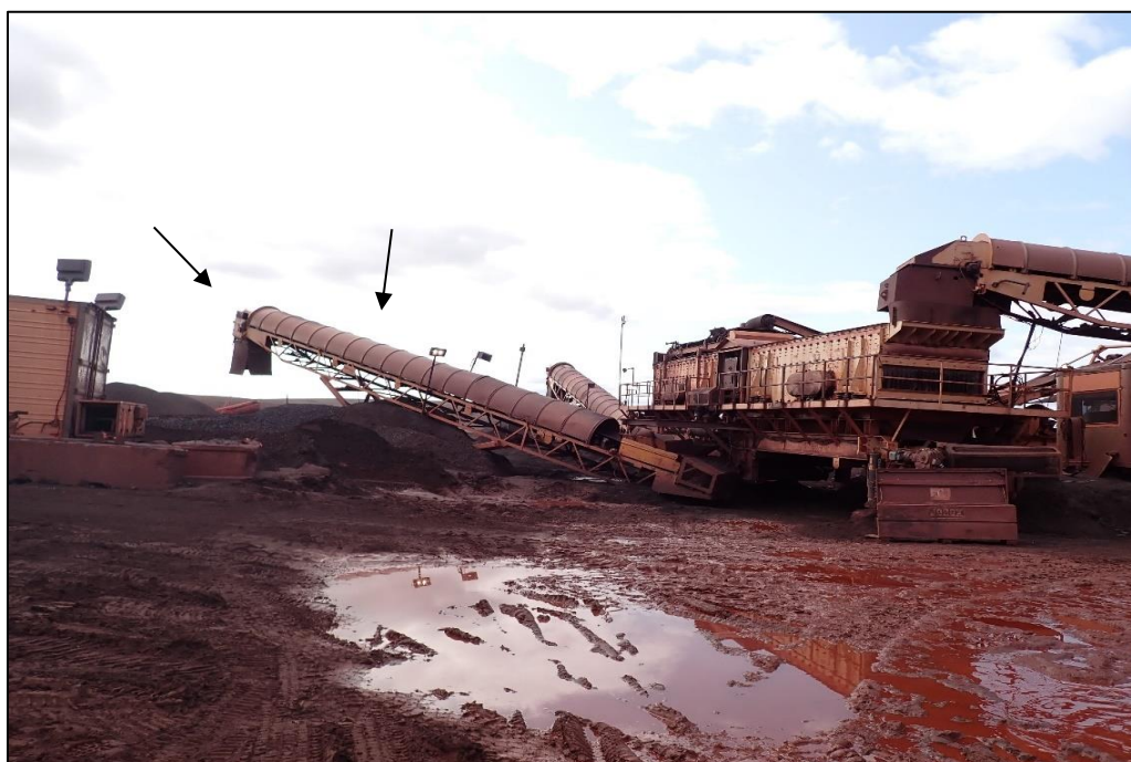
Photo 12: Hoods and Shrouding on Crusher Conveyor
