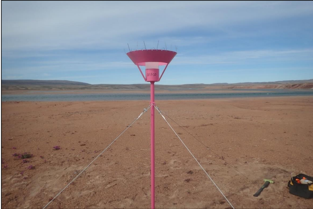
Photo 83: One of the New Dust Collectors around Milne Port
