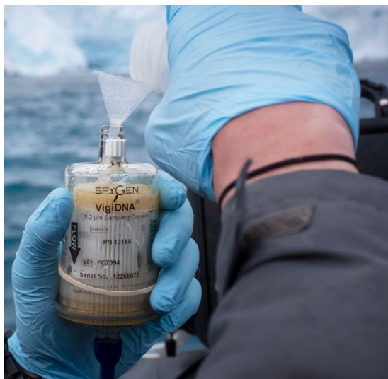
Figure 2 : Sampling capsule (provided by our partner SPYGEN). After sampling, these capsules need to be stored at room temperature in an upright position.
