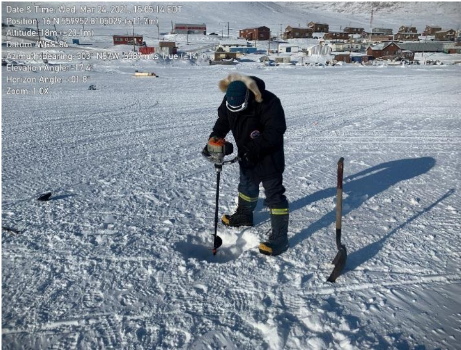
Photo 1 Augering hole through sea ice, March 24, 2021
