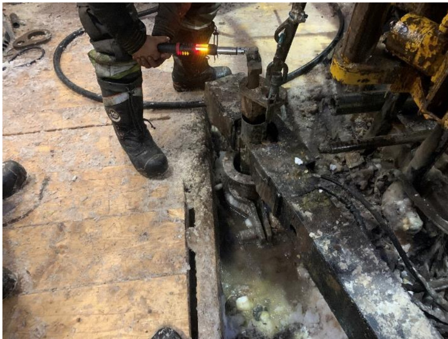
Photo 8 Field vane test at BH21-07, March 31, 2021
