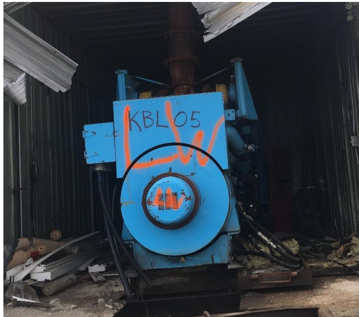
Photo 8. Prior to draining and flushing, each piece of equipment was marked with a unique identifier (i.e. KBL05). Following draining, flushing and inspection, each piece was signed off (i.e. LW) and marked ready as for disposal in the landfill.
