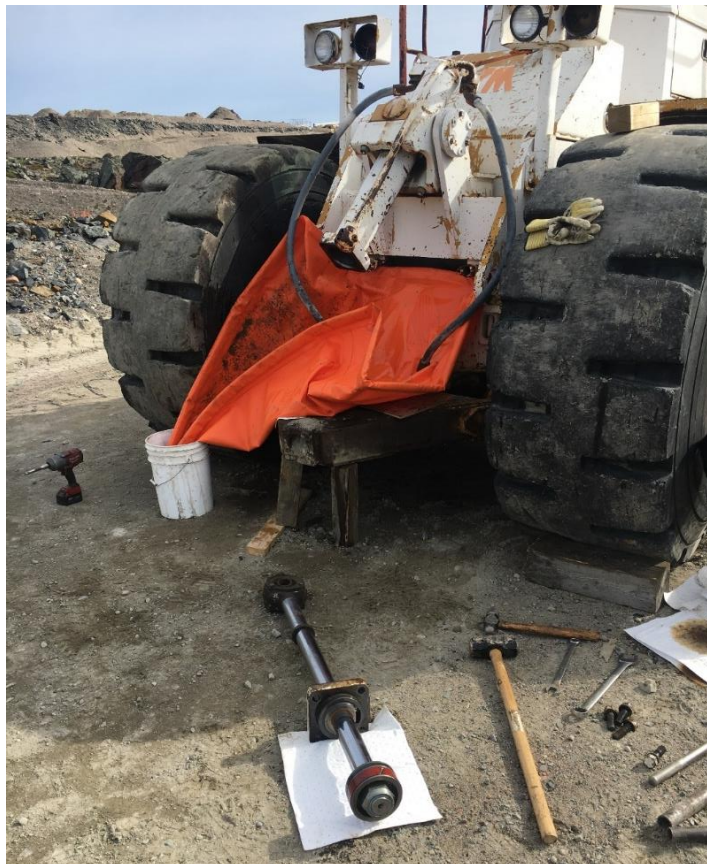
Photo 6. Equipment drained of fluids prior to disposal in the landfill
