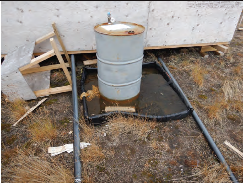
Description: secondary containment full of water.
