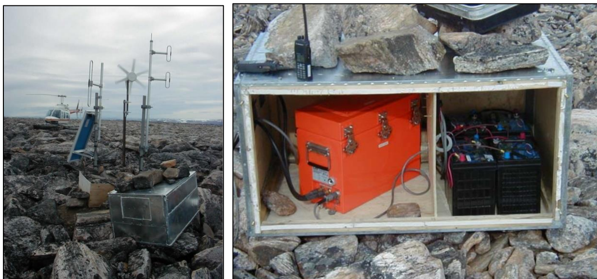
Figure 3. Qorbignaluk repeater site (left); Tuluria's battery array and transmitting equipment (right).
