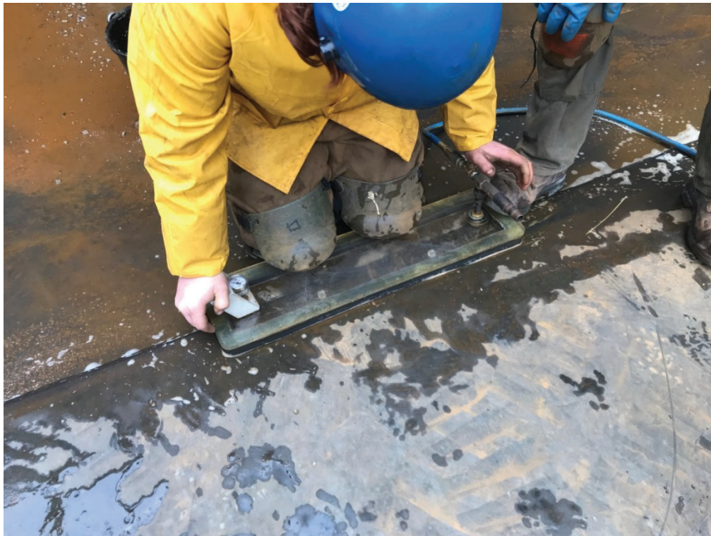
Weld testing with vacuum
