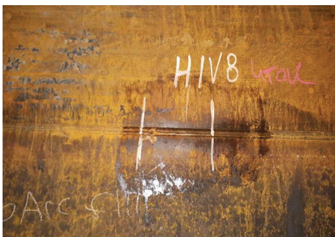
Photo #5: Typical horizontal spot (150mm length)
