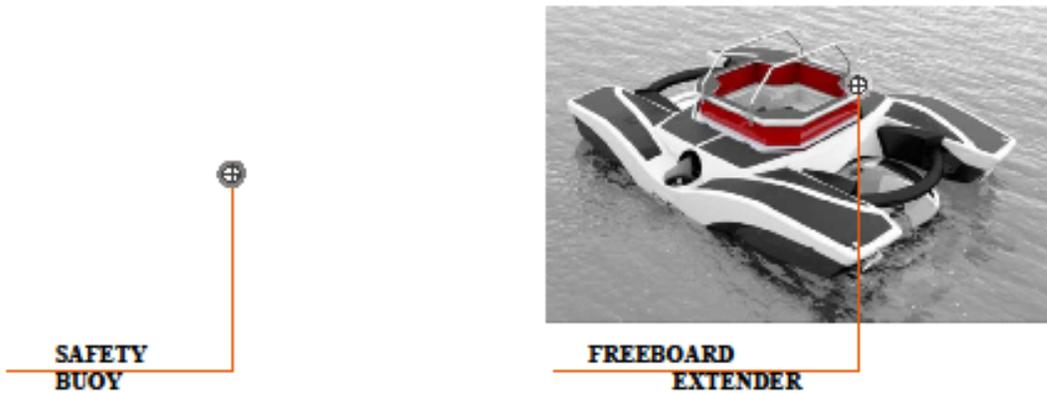
Freeboard is the height between the hatch and the waterline. The freeboard extender is a sliding barrier that increases the distance between the water and the hatch opening. It simultaneously allows for the submersible to be operated in rough conditions and be stored in low-height garage spaces.
