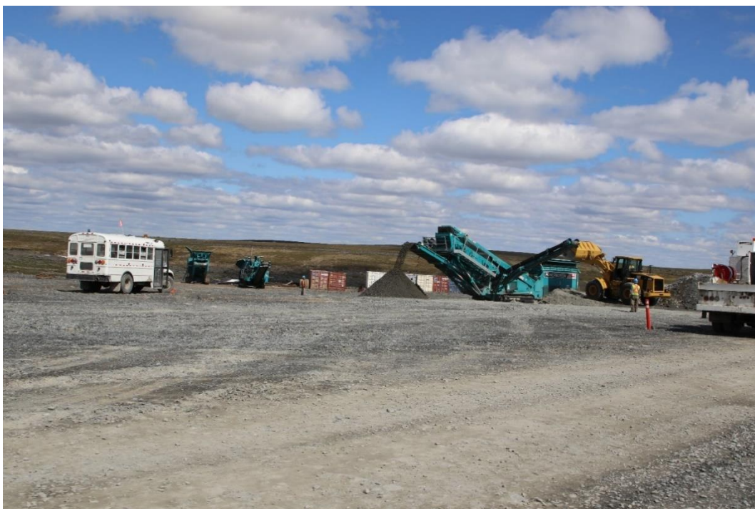
Photo 25: Crusher for Construction Material
