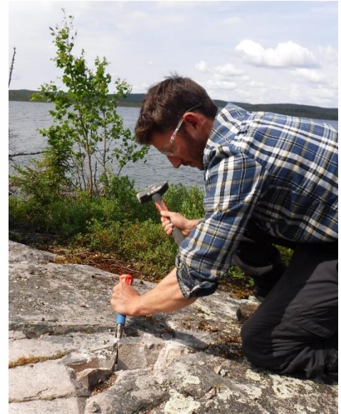
Rock sampling using a hammer and chisel.
