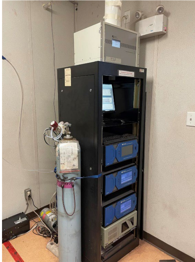
Photo 1.8 The rack-mounted Teledyne T100 ( \text{SO}_2 ) and T200 ( \text{NO}_x\text{-NO}_2 ) continuous gas analyzers at the PSC. The BAM 1020 analyzer for TSP is at the top of the rack.
