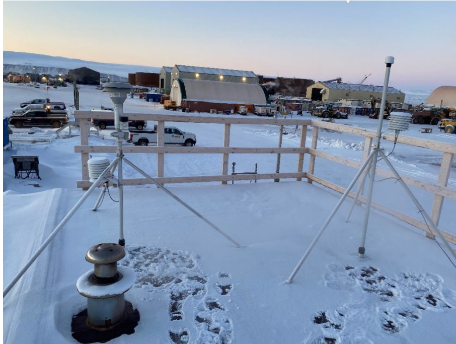
Photo 1.4 The TSP and PM 2.5 roof mount outlets and cutter heads.
