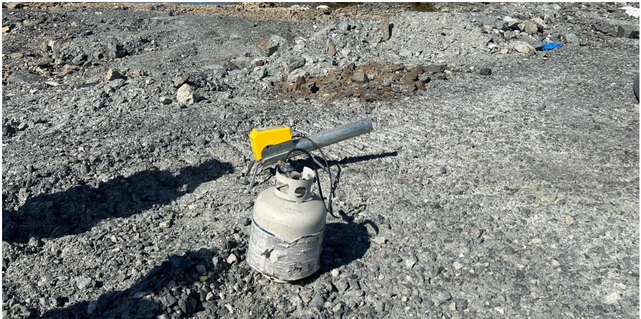
Photo 33: Wildlife deterrent or noise/bird cannon at the landfill site.
