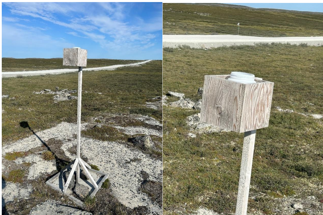
Photo 14: Close up images of dust monitoring equipment. The jars are removed and sent offsite for analysis.
