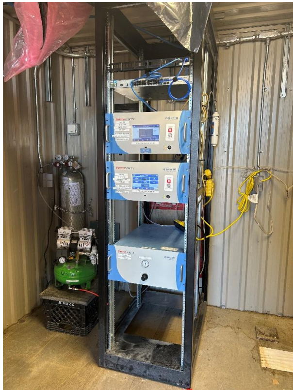
Photo 53 (left): Active NO 2 monitoring equipment with newly installed automatic shutoff switch to prevent equipment failure.
