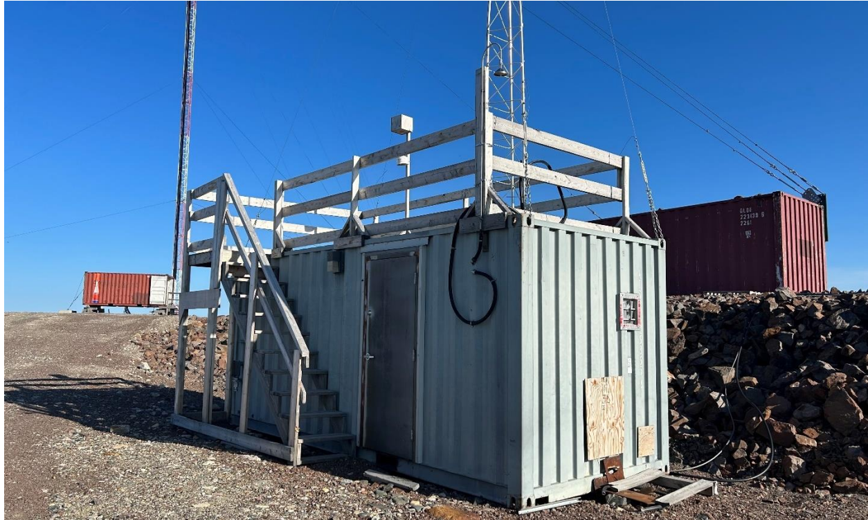
Photo 52: Sea-can housing the active NO 2 monitoring equipment. A Passive NO 2 monitor can be seen on the roof.
