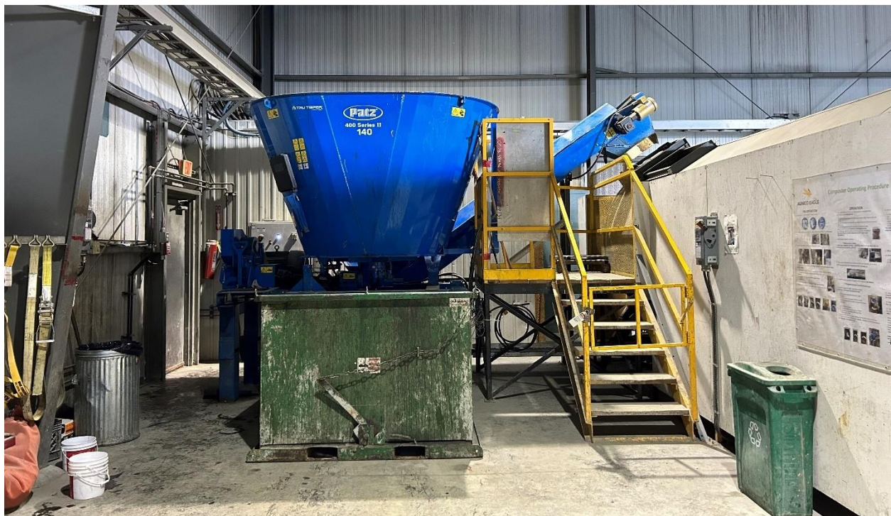
Photo 47: Composter at the Meadowbank Site. The Incinerator was previously housed in the same building but has since been removed due to exceedances during regular stack testing.
