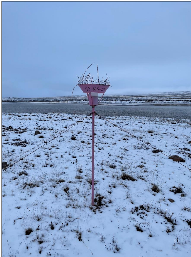
Photo 49: Passive Dust Sampler along the Tote Road
