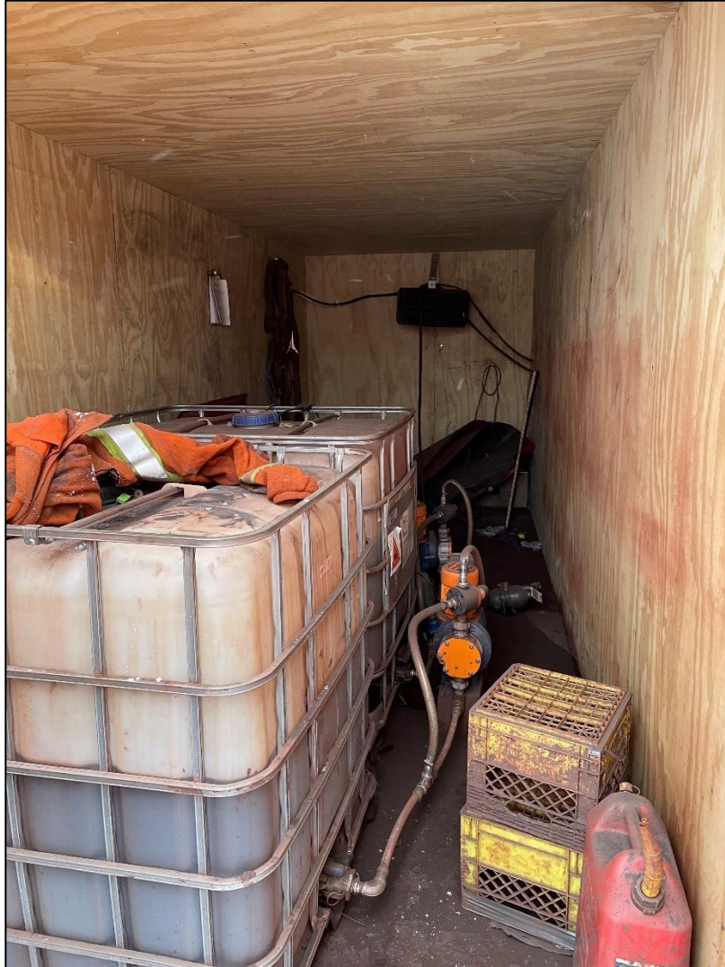
Photo 17: Liquid Dust Suppressant stored in a heated Seacan next to the crusher in preparation for the trial.
