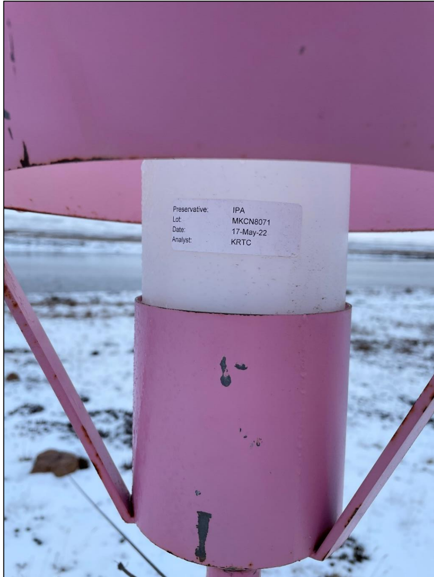
Photo 50: Close-up of Data Label on Passive Dust Sampler.
