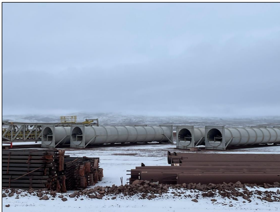
Photo 37: Enclosed Conveyor System Originally Procured for the Phase 2 Development Proposal.
