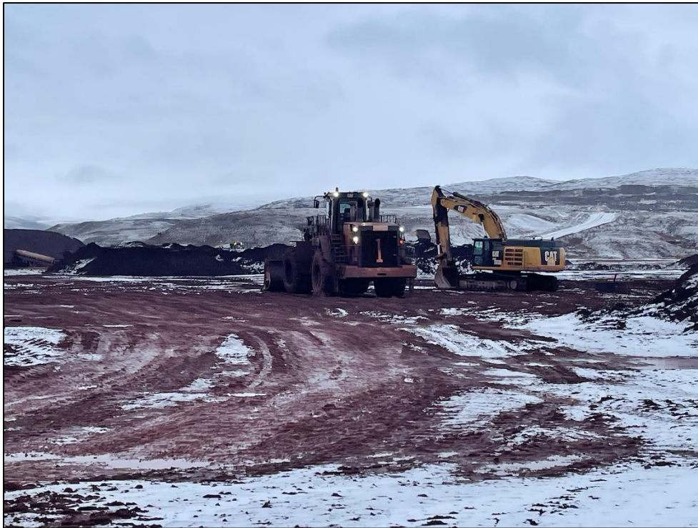
Photo 27: Loaders Moving Ore from the Stockpile to the Shiploader Conveyor.
