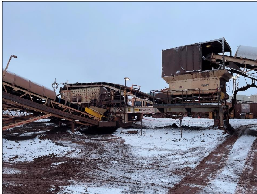
Photo 14: Hoods and Shrouds along the Crusher Conveyor.
