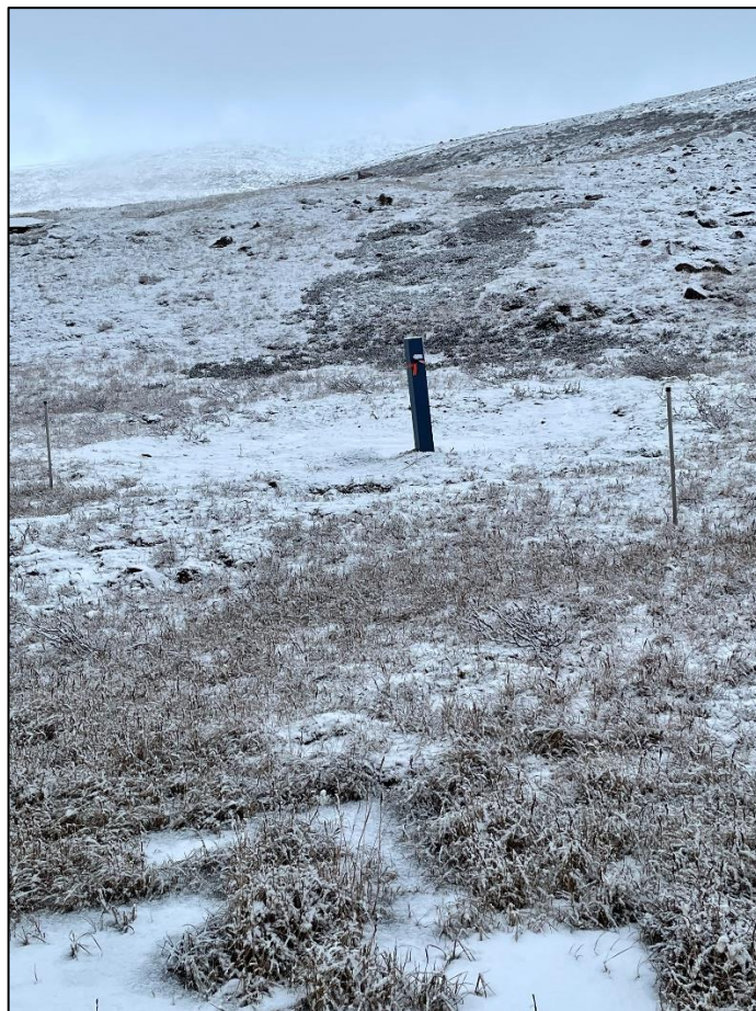
Photo 6: Groundwater Monitoring Station near the Landfill.
