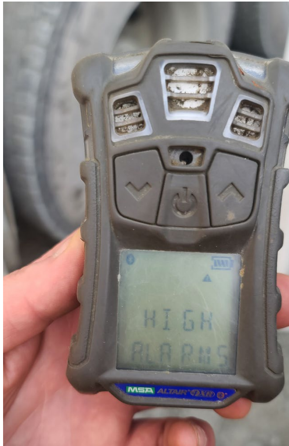
Figure 2. Underground air quality monitoring device.
