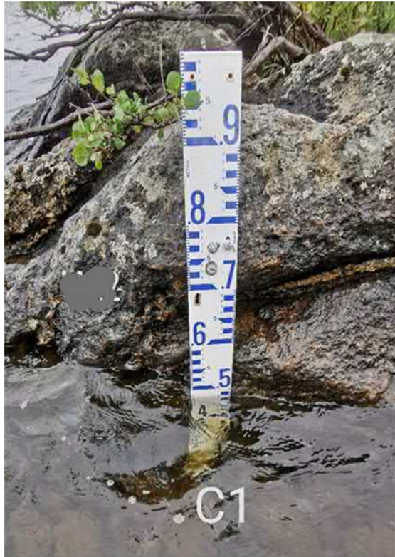
Figure 17: Example of a permanent, metal staff gauge as installed at station C1
