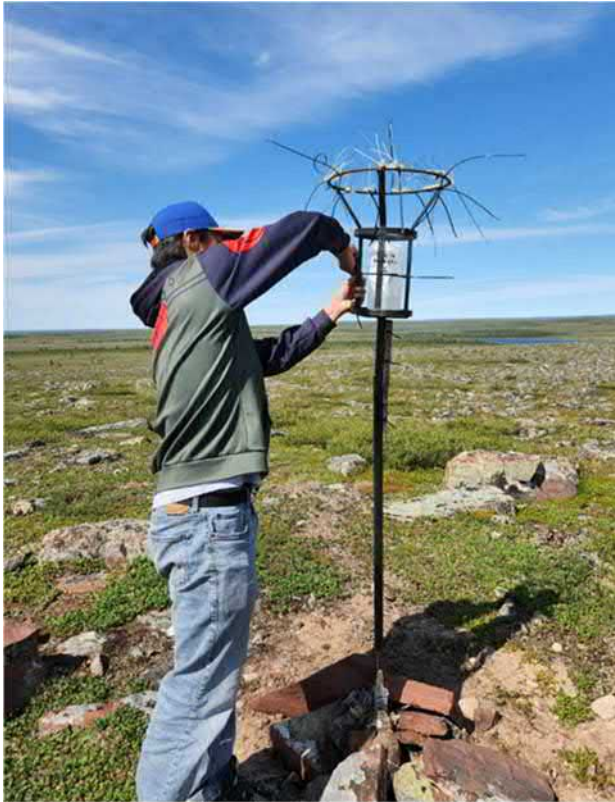
Figure 18: Installation of a fresh dust collecting canister at Dustfall Station DF1
