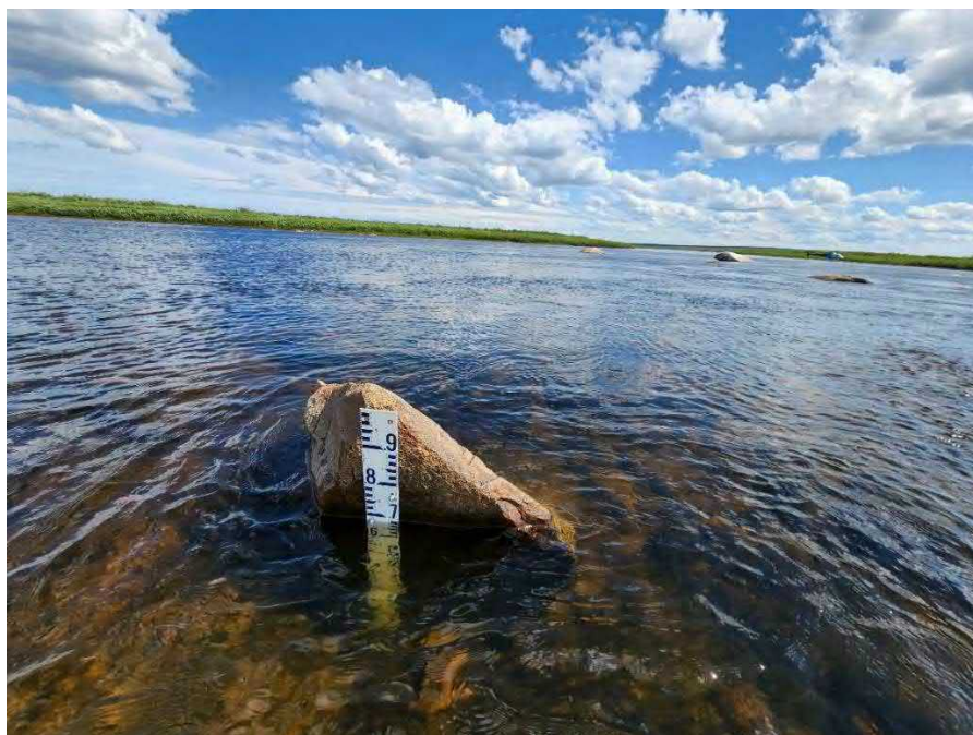
Photo 17 Established hydrology station S1.
