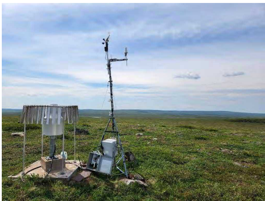
Photo 3 Rain gauge (left) alongside the climate station (right).
