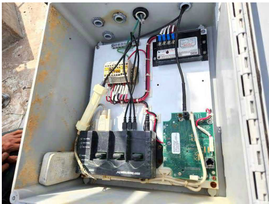
Photo 7 Inside logger box. HOB0 ONSET logger (black) shows significant corrosion damage as does the satellite communication chip (green).
