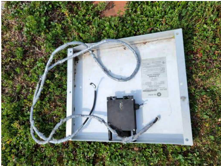
Photo 6 Climate station solar panel – wiring has been severed from station. Upon inspection the panel was not cracked but has been weathered and exposed to harsh climate for a prolonged period of time.
