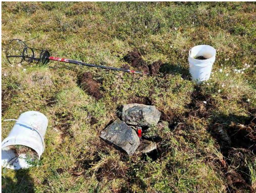
Photo 10 Dustfall installation process. Dug down to permafrost and laid a rock foundation. Station was then erected and as dirt / rock mound was laid for support.
