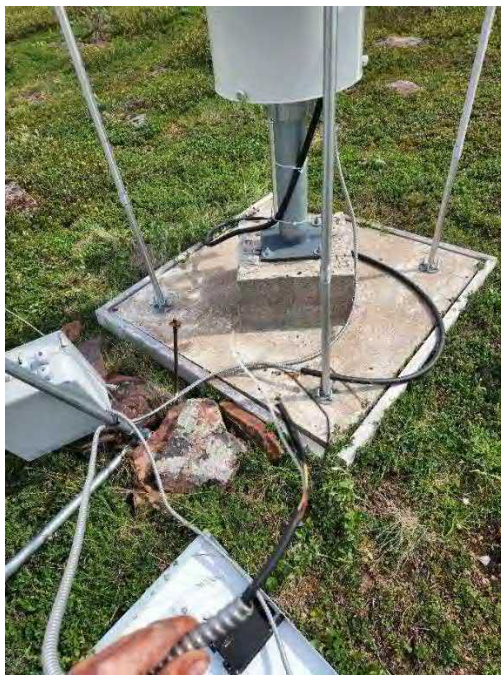
Photo 9 All logger sensor cables have been severed and destroyed over time.
