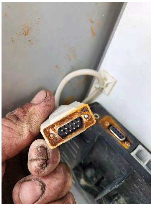
Photo 8 HOB0 logger corrosion from being exposed to elements over prolonged period of time.
