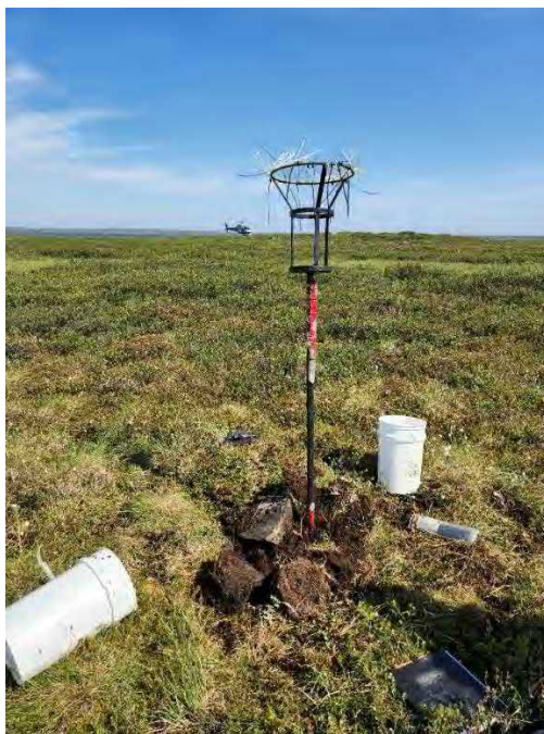
Photo 11 Erected dustfall station. Should the monitoring program continue, it is recommended that the stations be cemented in a 5-gallon pail and the pail be buried to permafrost.
