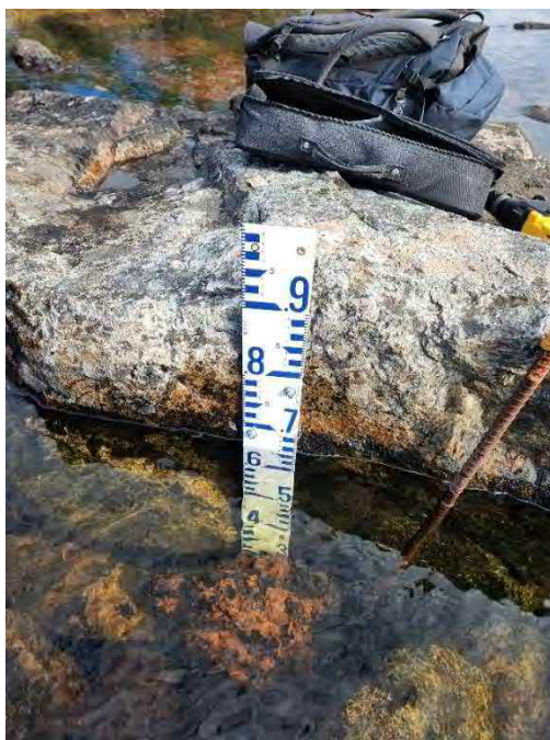
Photo 22 Established hydrology station W4.
