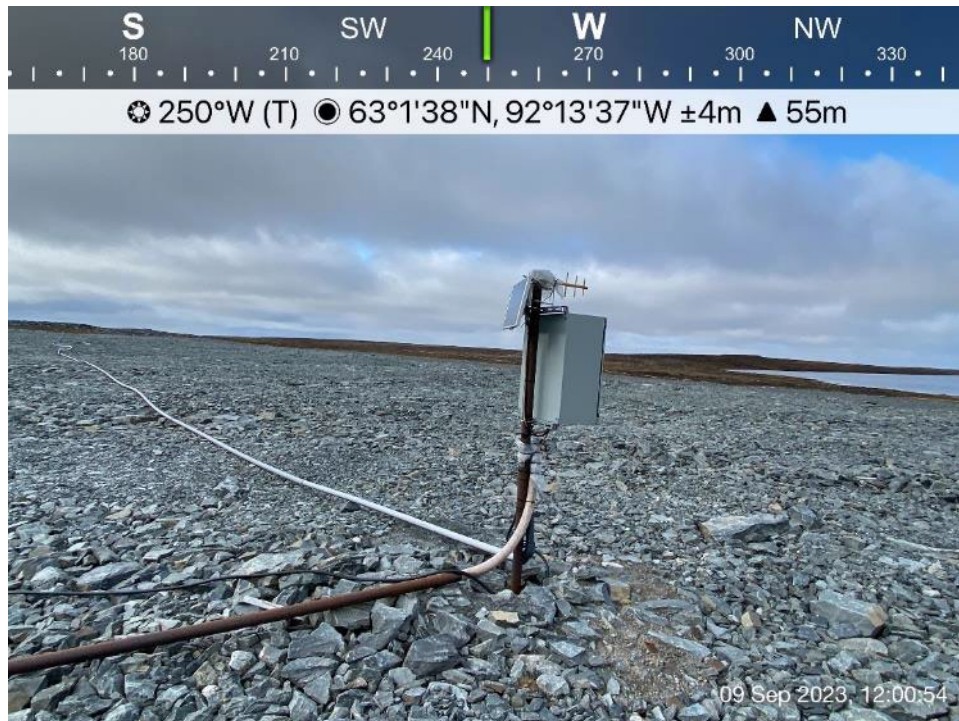
CP4 Thermal Berm - Photo 6: CP4 Thermal Berm - Looking west, GTCs data collection system.
