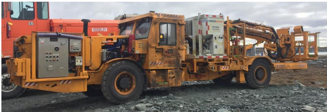
Figure 3-3 Underground Emulsion Charger – Dyno Loader
