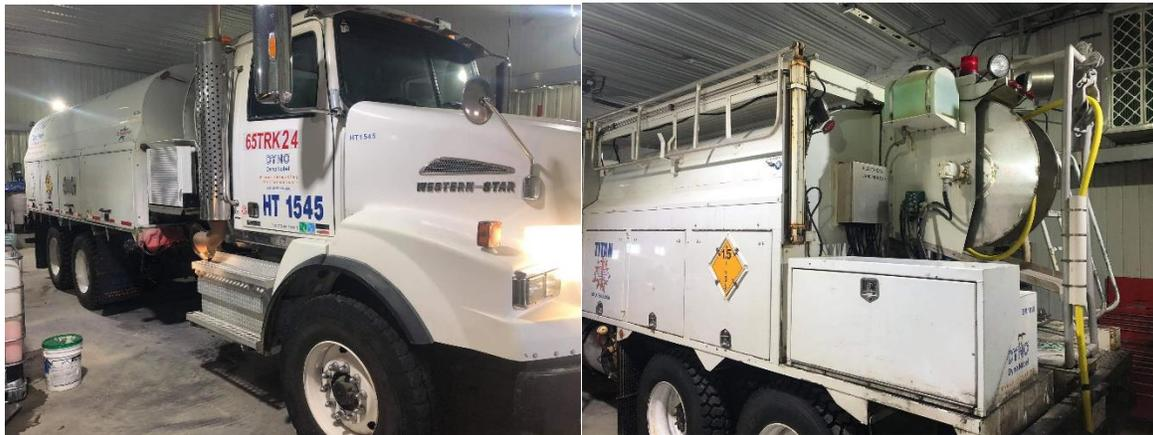
Figure 3-1 Mobile modular Emulsion Plant and Explosive Truck
