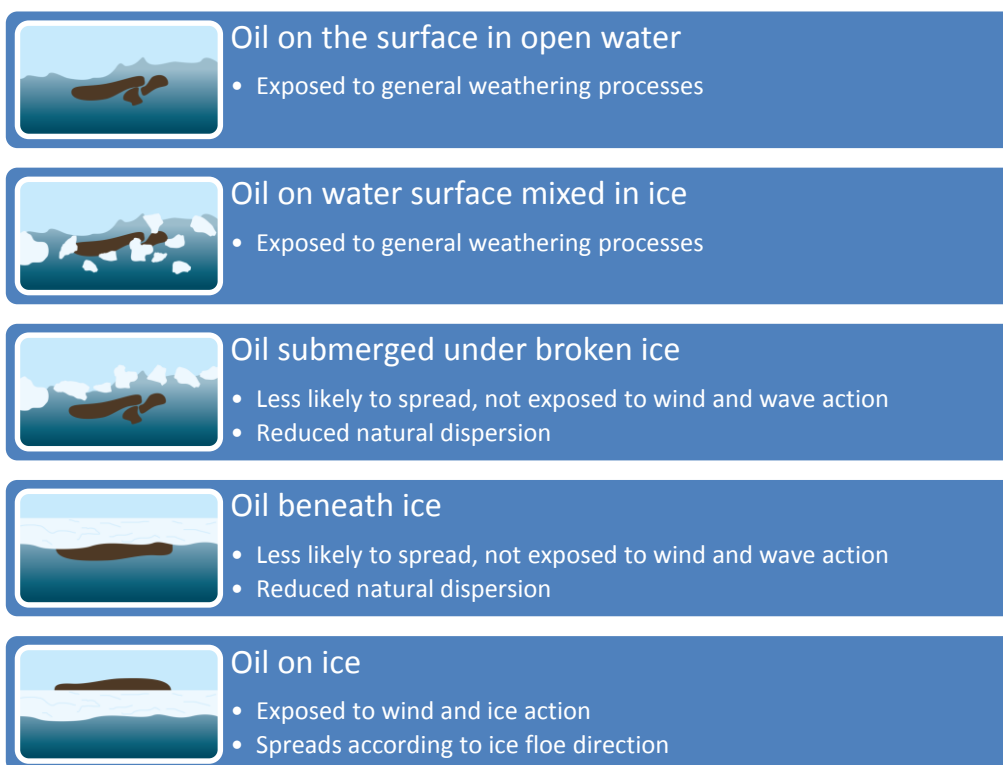
FIGURE 11-4: POTENTIAL FATES OF FUEL SPILLED IN COLD MARINE ENVIRONMENTS
