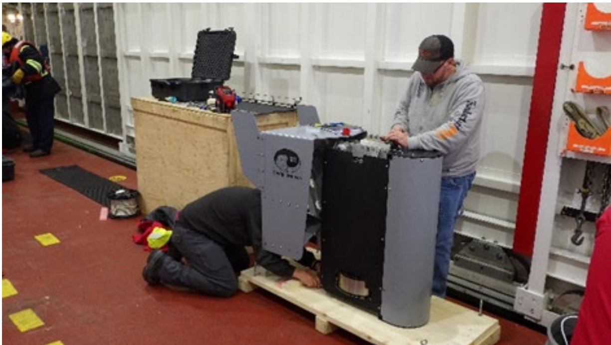
Photo 14 – Acoustic projector being setup for the Long Range Acoustic Communication Experiment
