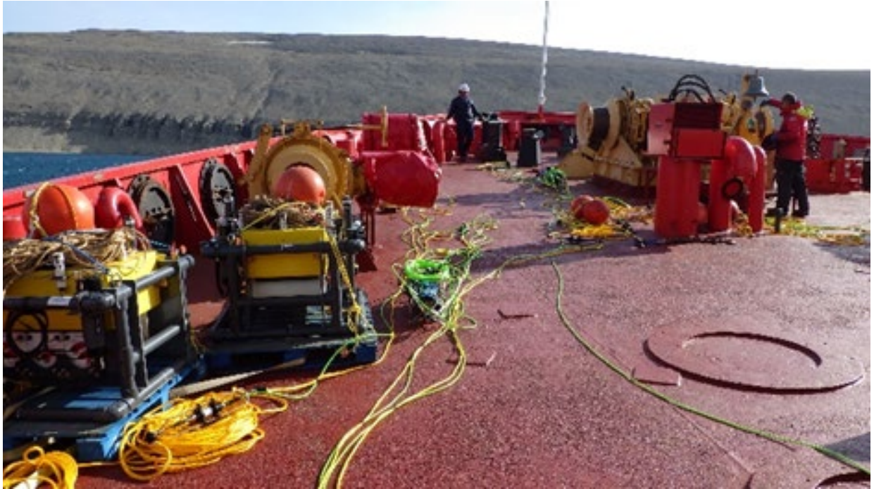
Photo 13 – Acoustic recorders for the Long Range Acoustic Communication Experiment (yellow/grey box units and blue units in left of frame)
