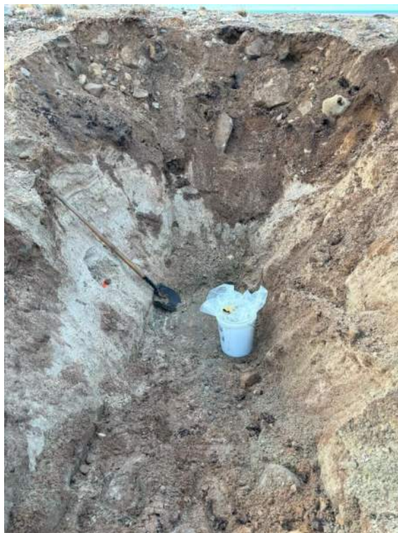
Photograph 25: Test Pit 5, Site 5, lower plateau. Note water in test pit.
