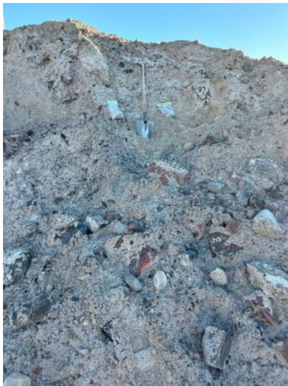
Photograph 31: Test Pit 7-1. Top of berm ridge, upper plateau, sand and gravel
