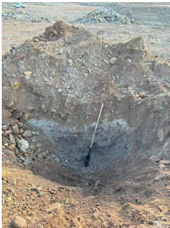
Photograph 5: Test Pit 2, Site 3, sand and gravel with cobbles and boulders
