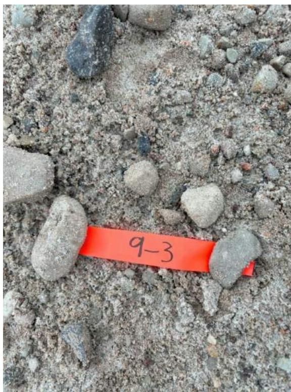
Photograph No. 41: Test Pit 3, Site 9, close up view of sample from test pit
