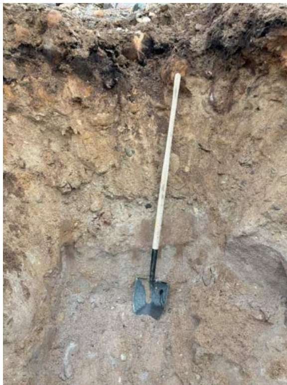
Photograph 7: Test Pit 3, Site 3, sand and gravel with cobbles
