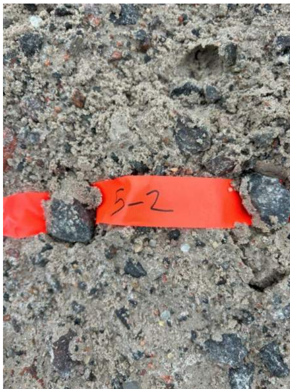
Photograph 24: Test Pit 2, Site 5, sand and gravel with cobbles and boulders
