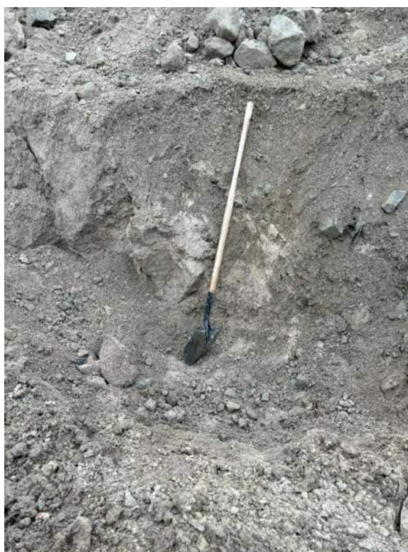
Photograph 34: Test Pit 3, Site 7. View of backfill in clay pit
