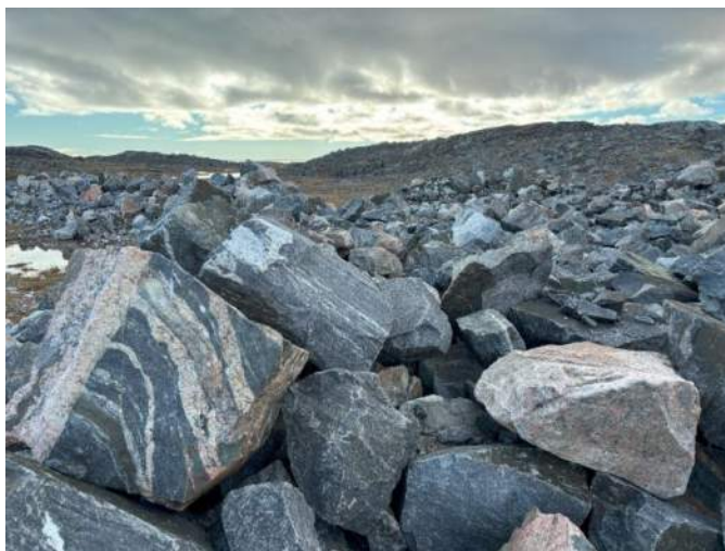
Photograph 4: Massive, oversized boulders, not crushable, stockpiled at quarry
