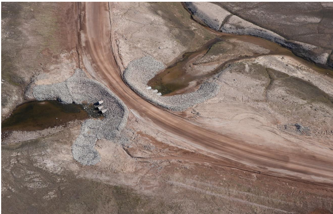
Photo 7: Completed Culvert Remediation along the Tote Road – June 2024
