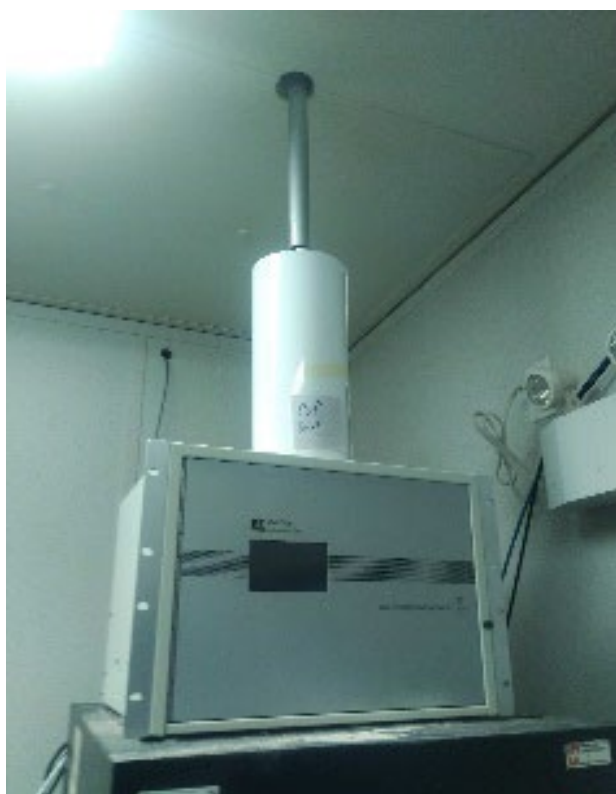
Photo 2.1 BAM 1020 for Continuous TSP Monitoring at the PSC – Nunami Stantec Limited.
