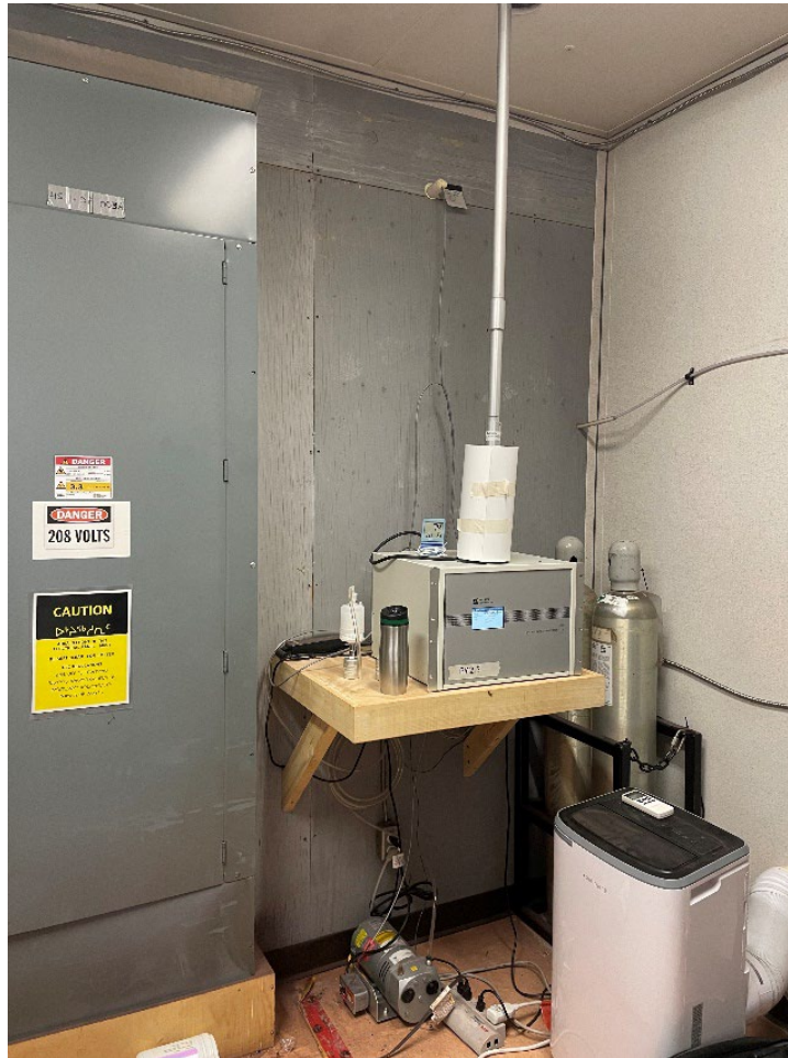
Photo 1.3 The PM 2.5 BAM analyzer at the MSC.
