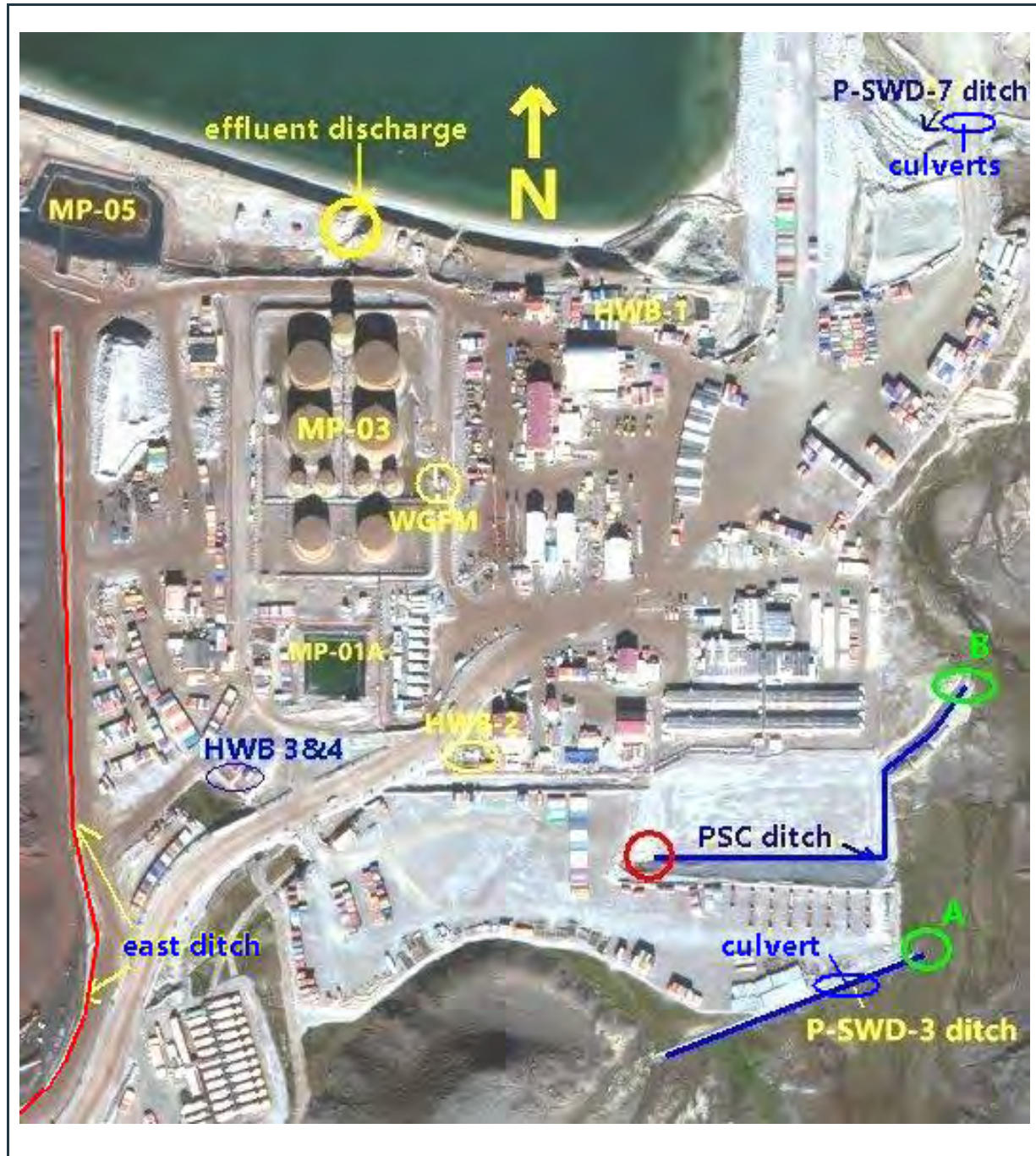
Figure 8: Site layout – Milne Inlet Port Site – North-Eastern Zone. © 2023 Digital Globe, Inc.
