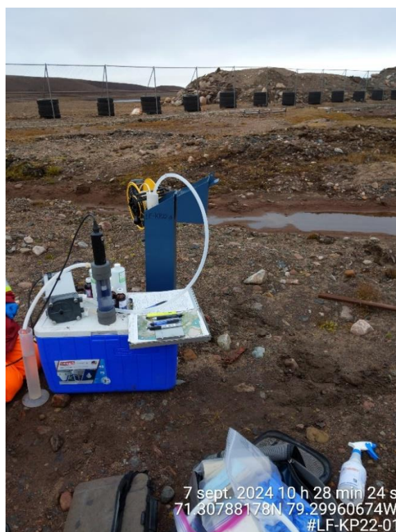
Photo A-19: Standpipe well LF-KP22-01 (7 September 2024) – Groundwater sampling set-up. A field blank was collected at this station.
