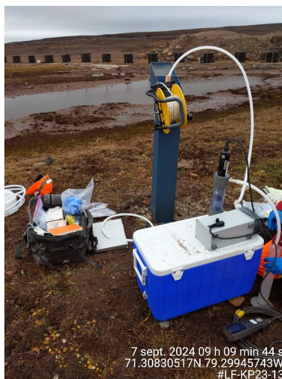
Photo A-18: Standpipe well LF-KP23-13 (7 September 2024) – Groundwater sampling set-up
