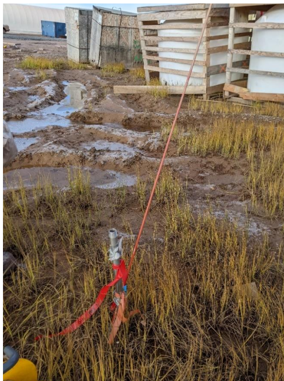
Photo A-6: Drive point piezometer MS-HWB-GW-REF3 (5 September 2024) – Collecting water level measurement and depth to well bottom using a water level tape.
