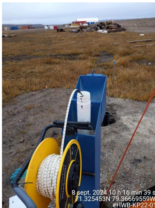
Photo A-28: Standpipe well HWB-KP22-01 (8 September 2024) – Collecting static water level prior to purging.
