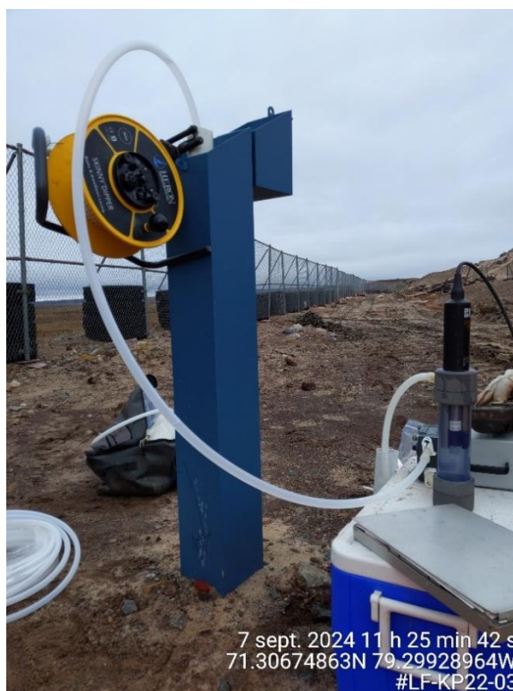
Photo A-20: Standpipe well LF-KP22-03 (7 September 2024) – Groundwater sampling set-up.
