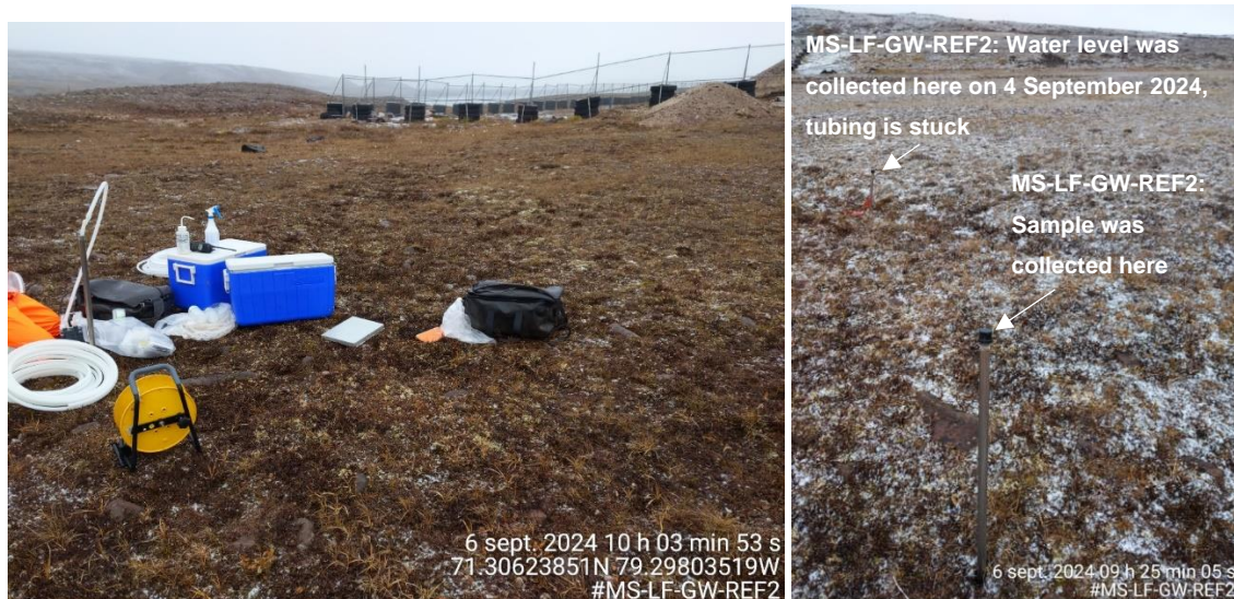
Photo A-14: Drive point piezometer MS-LF-GW-REF2 (6 September 2024) – Groundwater sampling set-up and 2 nearby drivepoints.
