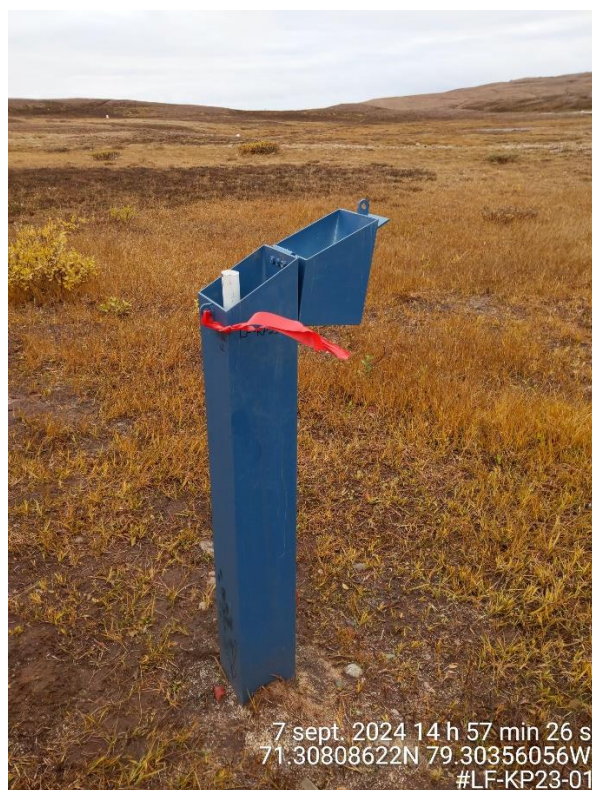
Photo A-27: Standpipe well LF-KP23-01 (7 September 2024) – Collecting static water level prior to purging.
