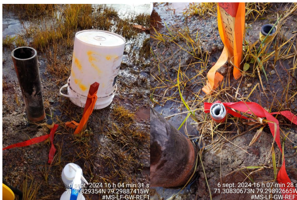
Photo A-17: Drive point piezometer MS-LF-GW-REF1 (6 September 2024) – Tubing is stuck in drivepoint, unable to collect a sample.
