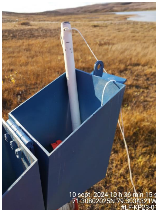
Photo A-47: Standpipe well LF-KP23-01 (10 September 2024) – Slug test was completed using a 0.30 m long and 0.75-inch diameter slug.
