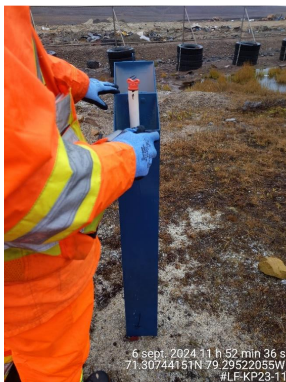
Photo A-16: Standpipe well LF-KP23-11 (6 September 2024) – Collecting static water level measurement prior to purging.
