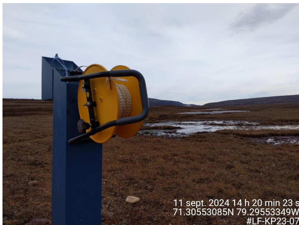
Photo A-53: Standpipe well LF-KP23-07 (11 September 2024) – Slug test set-up.
