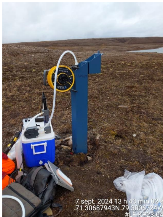
Photo A-23: Standpipe well LF-KP23-04 (7 September 2024) – Groundwater sampling set-up.
