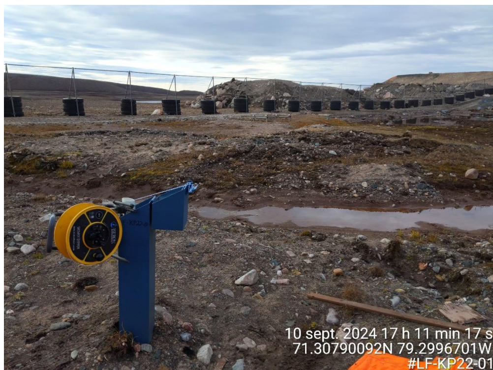
Photo A-50: Standpipe well LF-KP22-01 (10 September 2024) – Slug test set-up.
