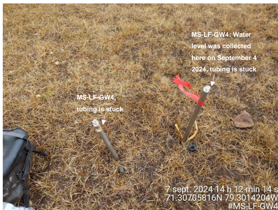
Photo A-24: Drive point piezometer MS-LF-GW4 (7 September 2024) – Tubing is stuck at both nearby drive point piezometers, unable to collect a sample at this station.
