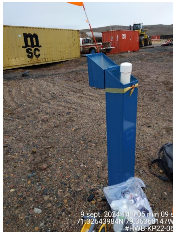
Photo A-39: Standpipe well HWB-KP22-06 (9 September 2024) – Well was dry, no sample collected.
