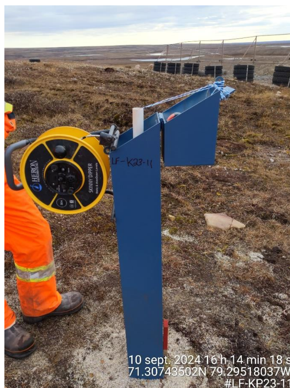
Photo A-49: Standpipe well LF-KP23-11 (10 September 2024) – Slug test set-up.
