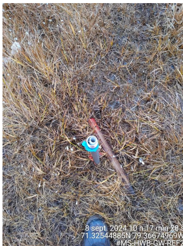
Photo A-29: Drive point piezometer MS-HWB-GW-REF2 (8 September 2024) – Tubing is stuck, unable to collect a sample at this station.
