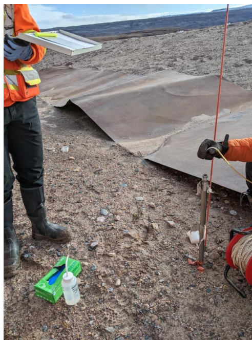
Photo A-7: Drive point piezometer MS-HWB-GW3 (5 September 2024) – Collecting water level measurement and depth to well bottom using a water level tape.
