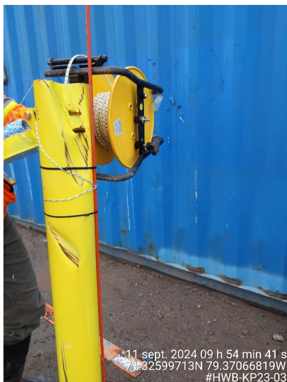
Photo A-51: Standpipe well HWB-KP23-03 (11 September 2024) – Slug test set-up.
