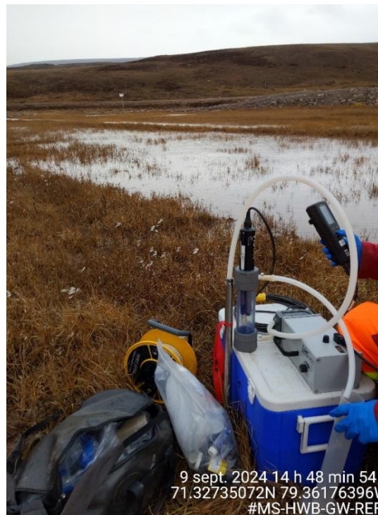
Photo A-40: Drive point piezometer MS-HWB-GW-REF1 (9 September 2024) – Groundwater sampling set-up. Standing water around the station. No cap was on the drive point piezometer prior to sampling, and it had been raining in the days prior to collecting sample. A cap was installed after sampling completed.
