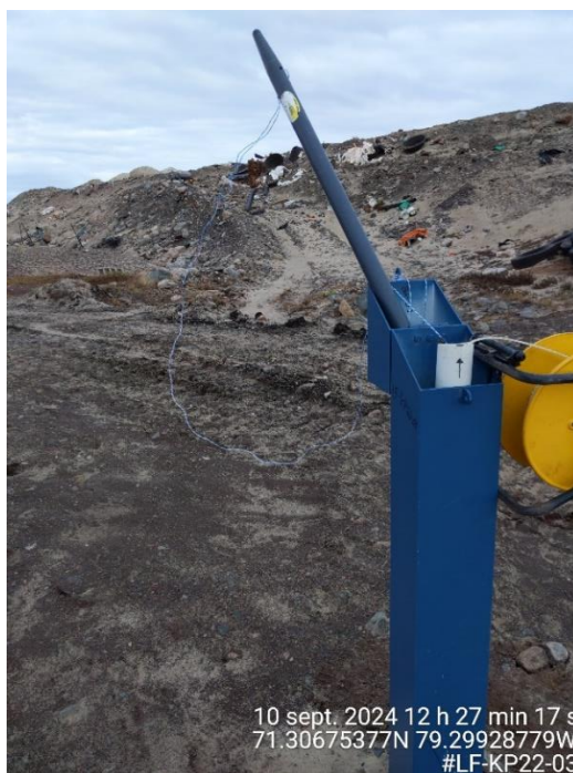
Photo A-48: Standpipe well LF-KP22-03 (10 September 2024 – Slug test was completed using a Midwest Geoscience slug of 0.92 m long and 1.5-inch diameter.
