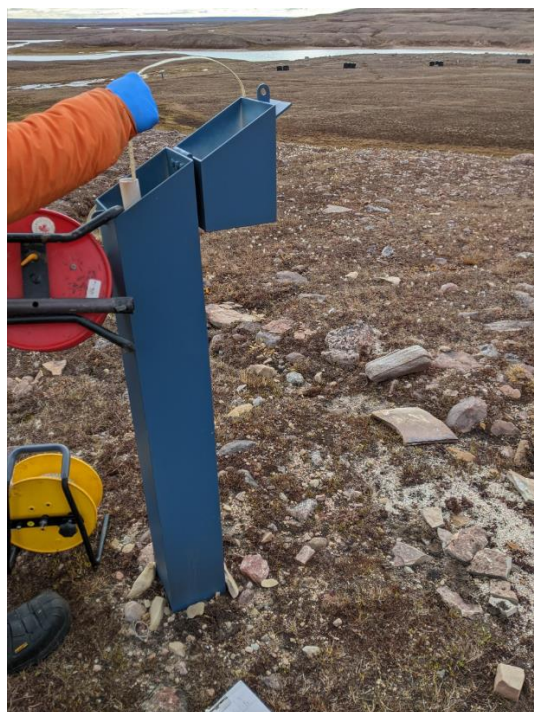
Photo A-3: Standpipe well LF-KP23-10 (4 September 2024) – Collecting water level measurement and depth to well bottom using a water level tape.
