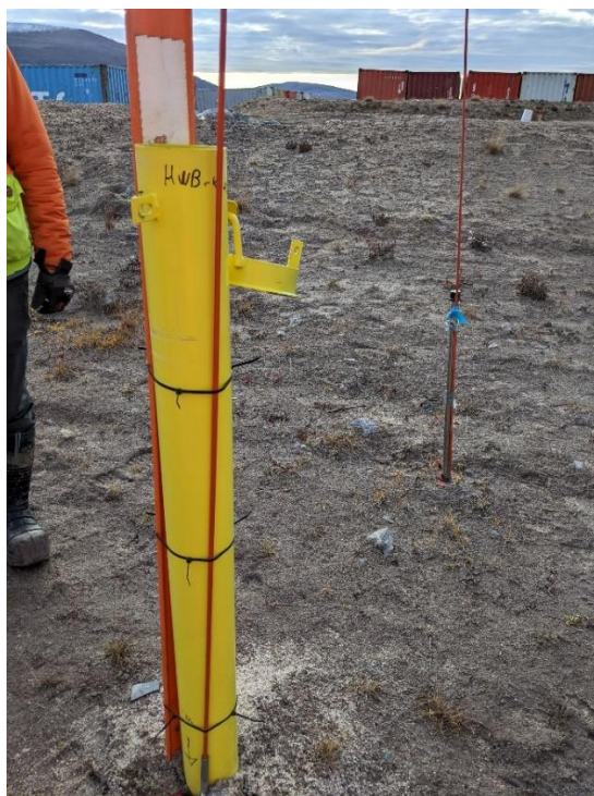
Photo A-5: Standpipe well HWB-KP23-01 (5 September 2024) – Collecting water level measurement and depth to well bottom using a water level tape.
