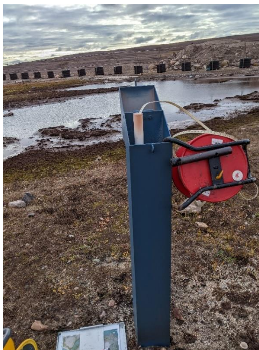
Photo A-2: Standpipe well LF-KP23-13 (4 September 2024) – Collecting water level measurement and depth to well bottom using a water level tape.
