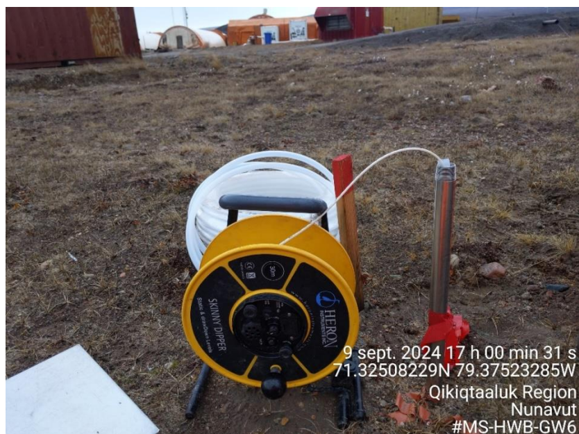
Photo A-41: Drive point piezometer MS-HWB-GW6 (9 September 2024) – Station was dry, no sample collected.
