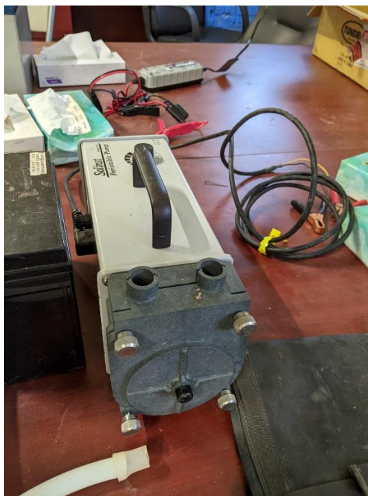
Photo A-10: Solinst Peristaltic Pump (Model 410) used for purging and collecting groundwater samples.
