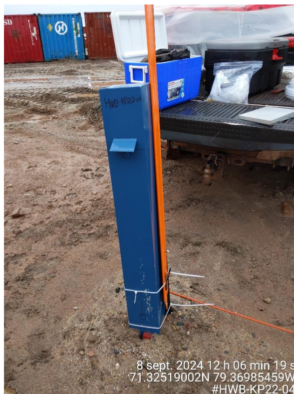
Photo A-31: Standpipe well HWB-KP22-04 (8 September 2024) – Groundwater sampling set-up.
