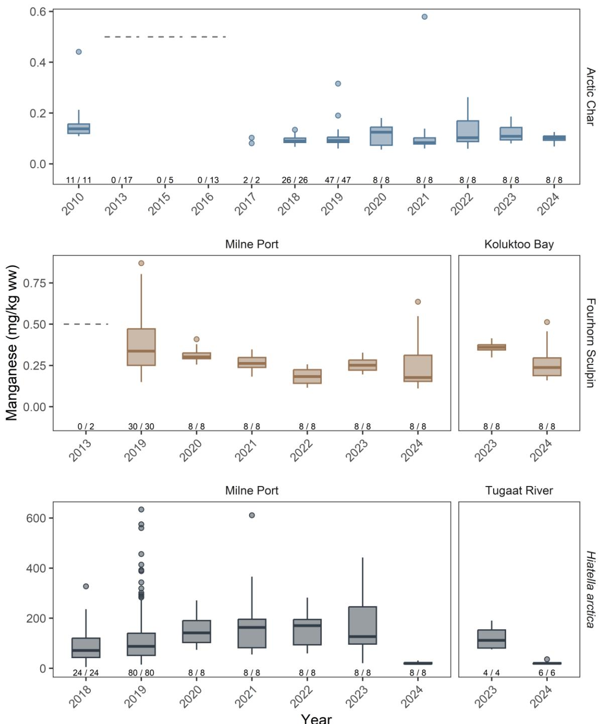
Total sample size (n) and number of samples above detection limits (n>DL) are shown above the x-axis as “n>DL/n”. Values below DL are not shown in the plots. Dashed lines indicate detection limits.
