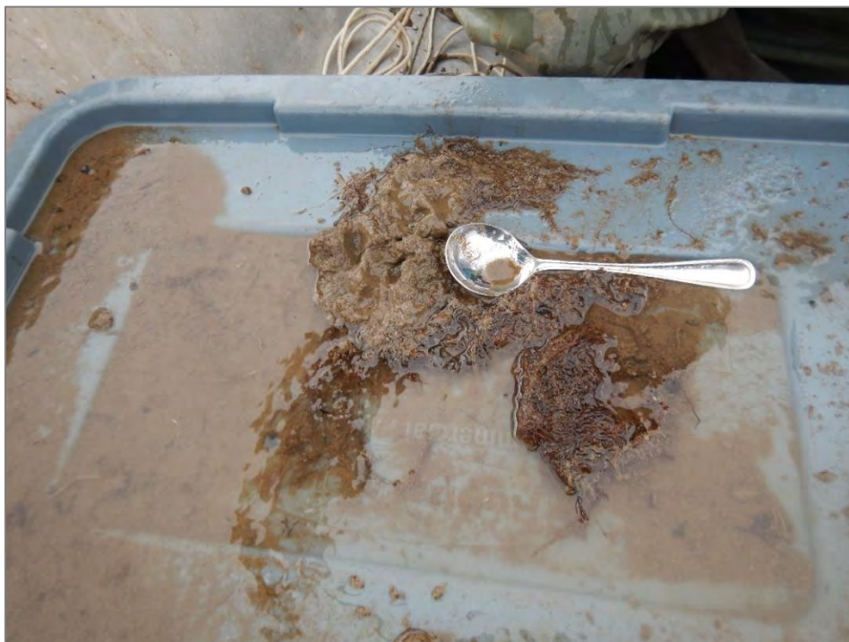
Photograph 7. Silt/clay substrate with organics sampled with a petite Ponar dredge sampler (Site 10).
