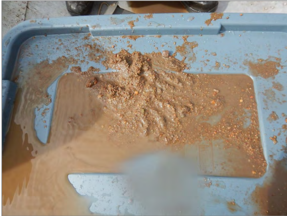
Photograph 4. Sandy gravel substrate sampled with a petite Ponar dredge sampler (Site 23).
