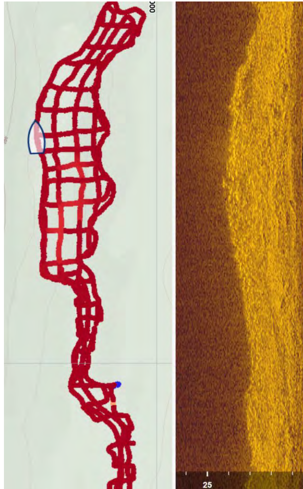
Figure 4. Sidescan image data showing cobble and boulder substrate within 12-15 metres of the shallow western shore of the north basin of KP85 Lake.
