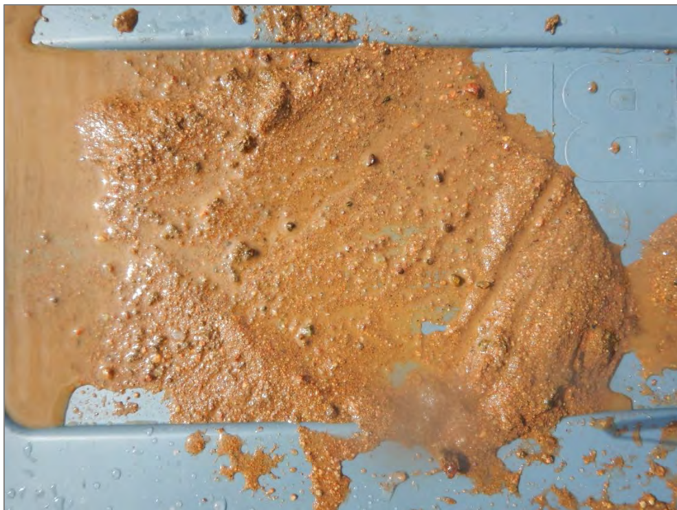
Photograph 5. Sand substrate sampled with a petite Ponar dredge sampler (Site 19).
