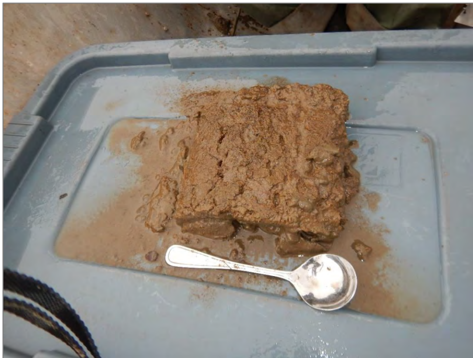
Photograph 6. Moderately compacted clay and silt substrate sampled with a petite Ponar dredge sampler (Site 32).
