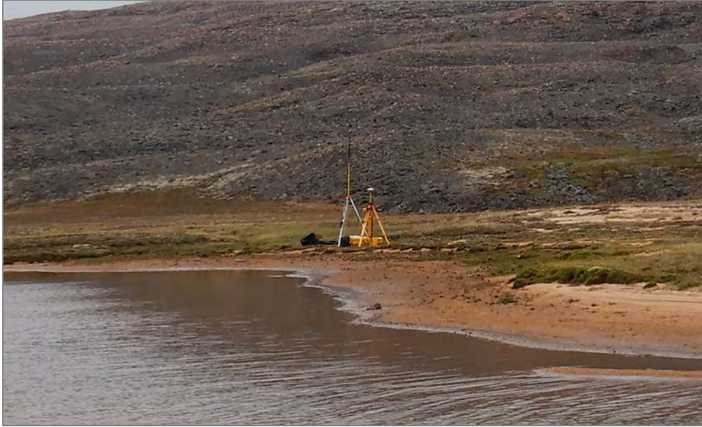
Photograph 1. RTK GNSS base station receiver setup along the sandy shores at the midpoint between the north and south basins of KP85 Lake.
