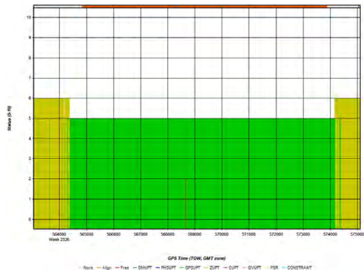
Figure 8: Aug10Flight1 [Smoothed TC Combined] - Status flag for IMU processing
