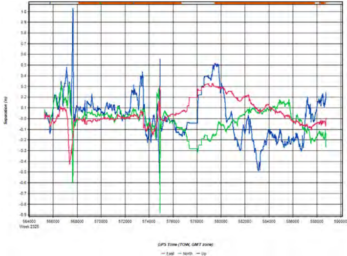
Figure 2: Aug3_Flight1 [Smoothed TC Combined] - Forward/Reverse or Combined Separation Plot
