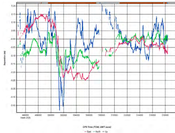
Figure 4: Aug2_Flight1 [Smoothed TC Combined] - Forward/Reverse Separation Plot (Fixed)
