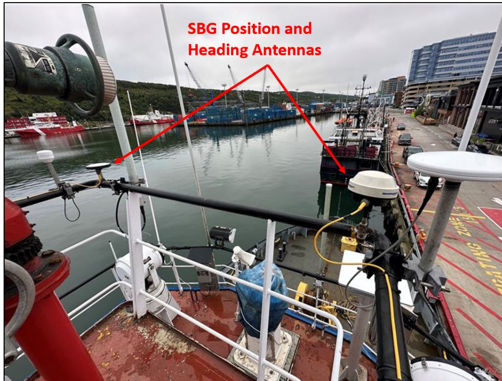
Figure 4-2: Location of SBG positioning and heading antennas on vessel superstructure.
