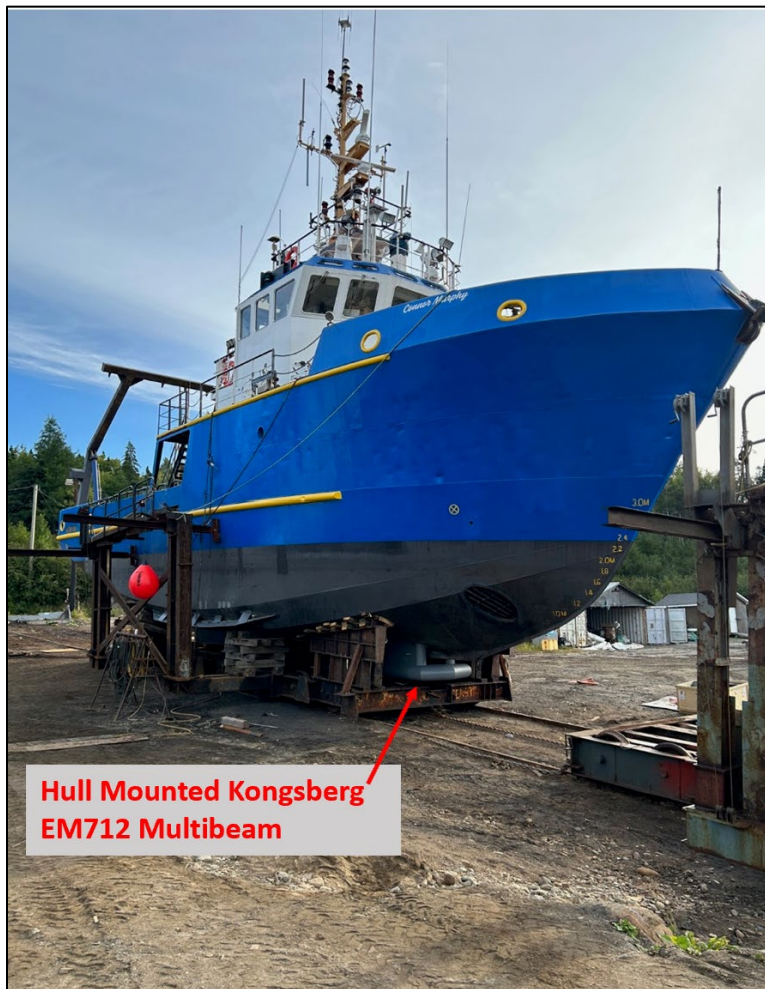
Figure 4-3: Hull mounted Kongsberg multibeam on the Connor Murphy
