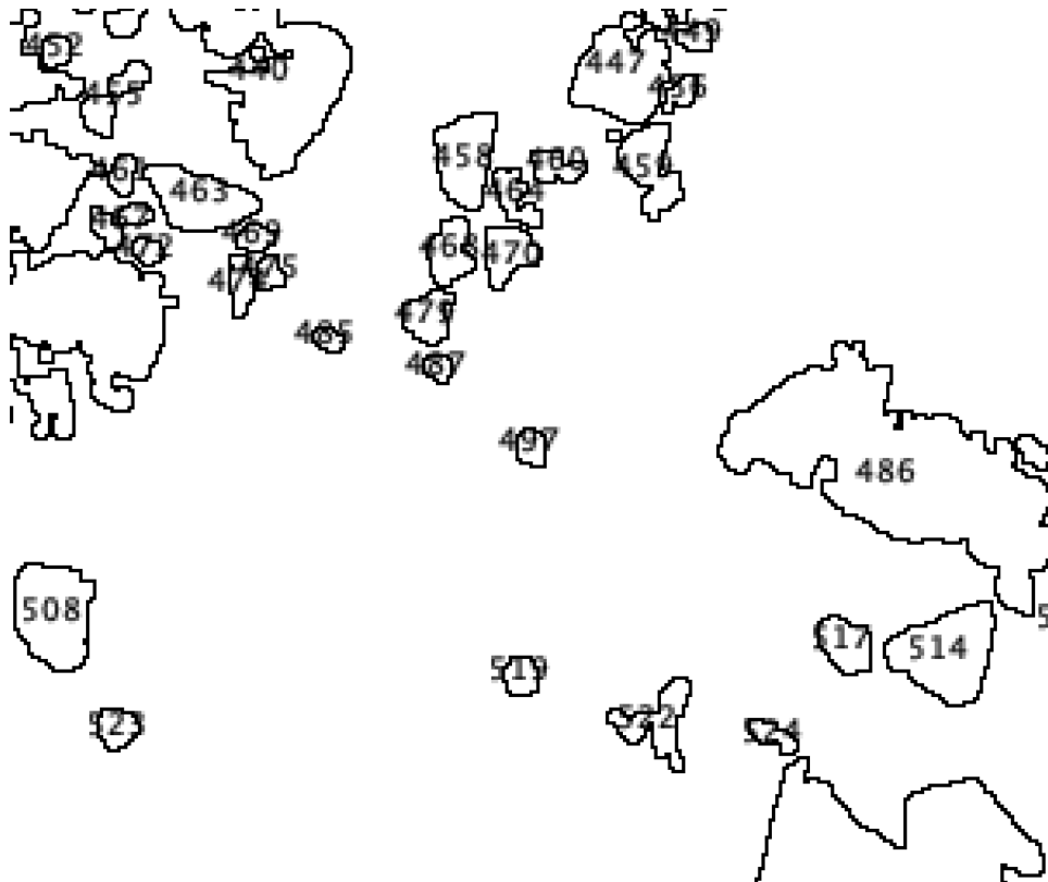
Figure 4: An extract of the particle analysis with identification and assignment of a unique identification number to each individual ice floe.
