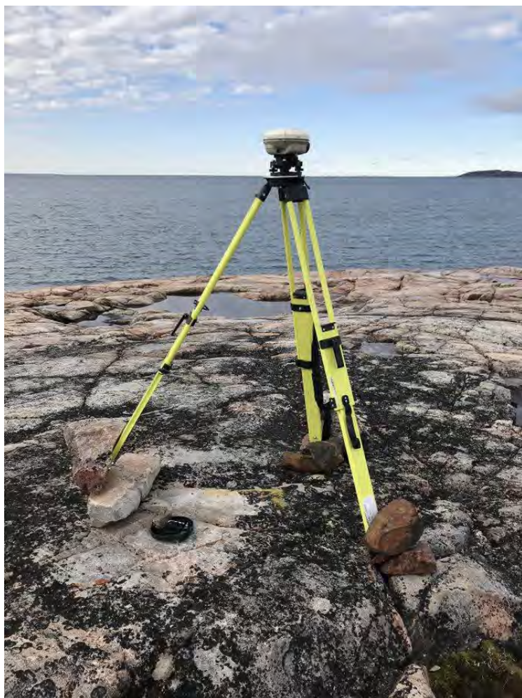
Photo 71: RTK Survey Local Ground Control Point base station set up 40 m inland above the Ore Dock (5 September 2021).
