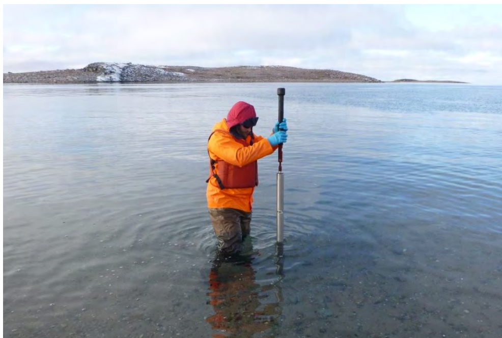
Photo 26: AMS Multi-Stage Corer attempting to collect sediment samples at the Causeway (14 September 2021).
