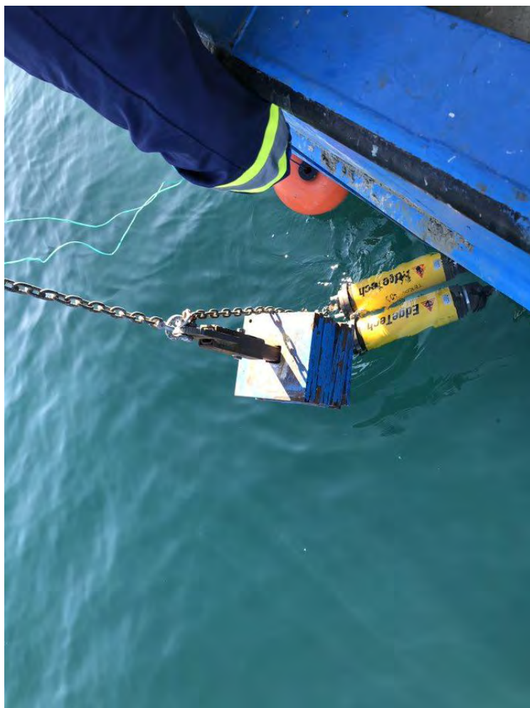
Photo 72: ACDP Mooring deployment to 78 m depth to the west of the Ore Dock (8 September 2021).
