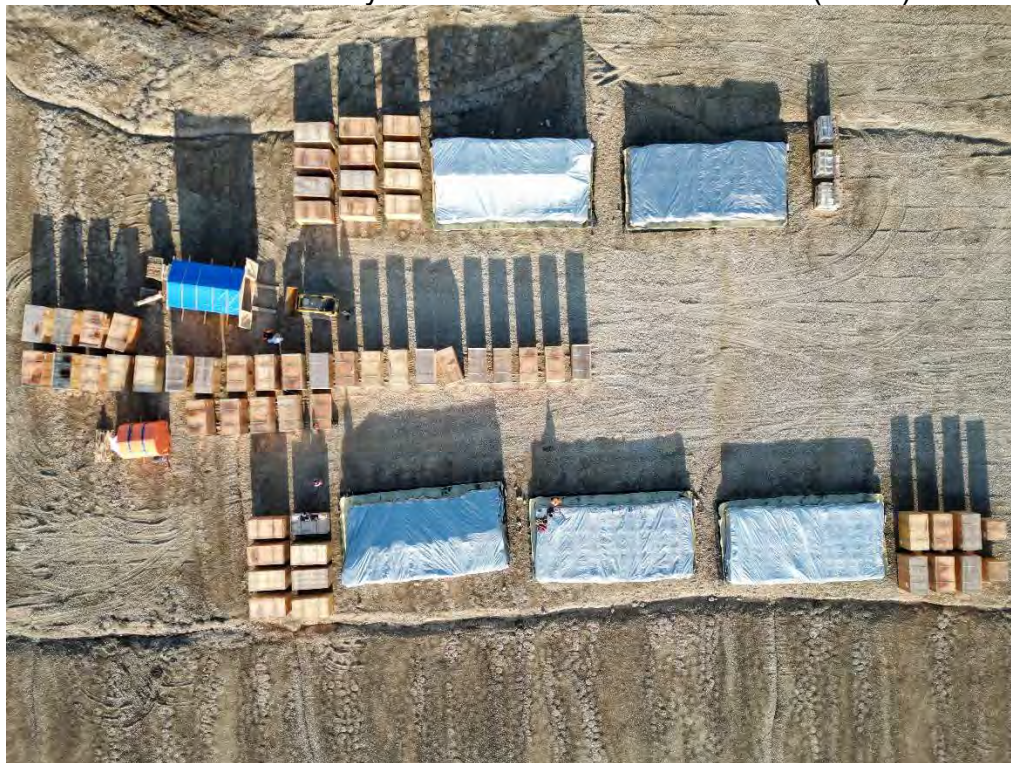
Photo 4. Sealift laydown with covered fuel berms (aerial)
