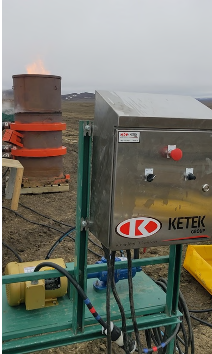
Figure 9: Waste fuel pump and control panel and burn chamber with ideal flame height shown
