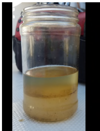
Figure 10: Fuel and Water separation in a glass
