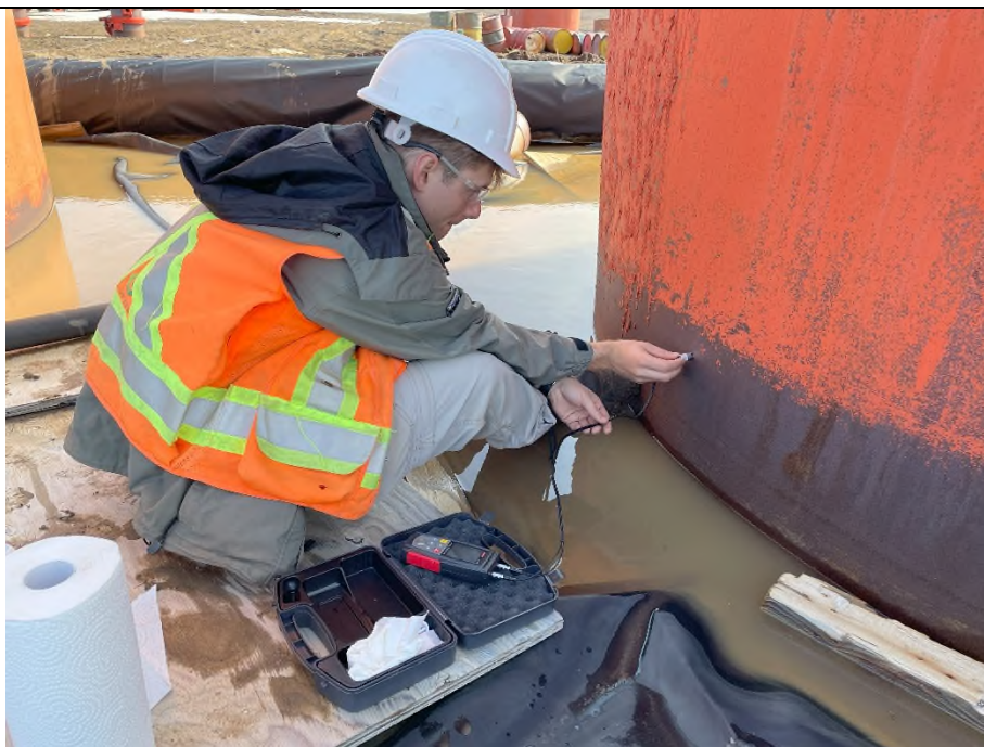
Photo 2: Measuring steel thickness of tanks using an Ultrasonic Velocity Meter, view South. (July 6, 2024)
