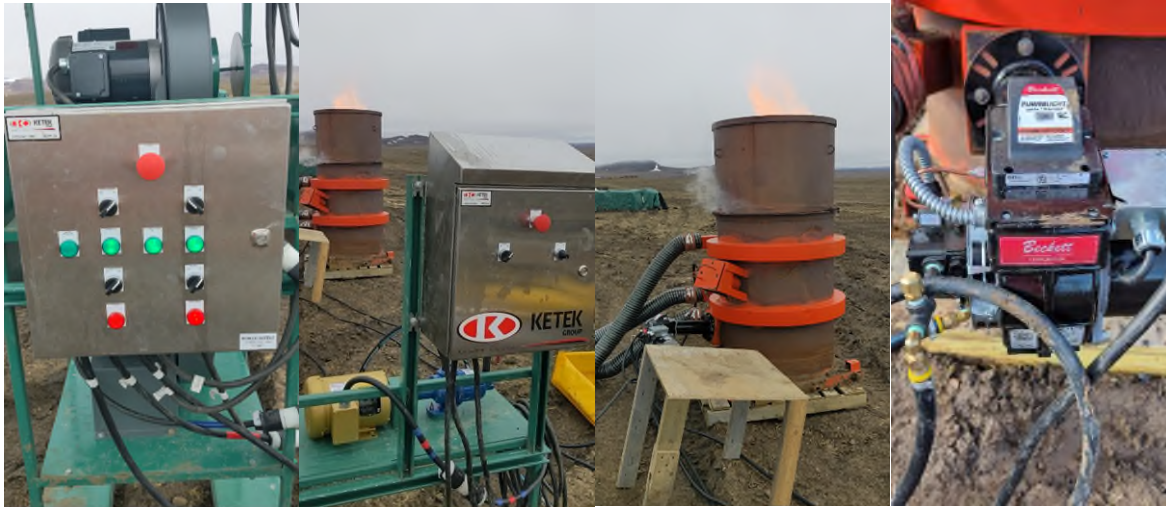
Figure 4: Clean Diesel and waste fuel for pilot burners (left), Proposed Mixing Tank (middle left), proposed oily water fuel separation tote (middle right) and proposed Field Generator (1 required for each incinerator setup) (right)
