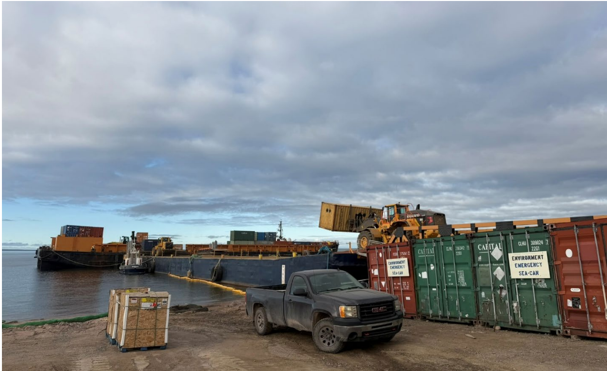
Photo 2: Loader handling seacan during barge unloading operations, with dedicated spill response seacans available for environmental protection and emergency response
