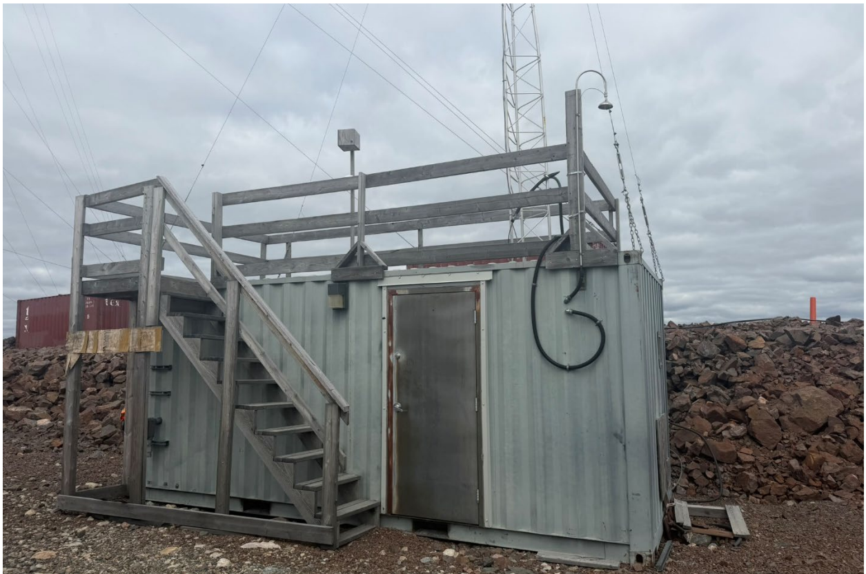
Photo 68: NO 2 monitoring station, with both active and passive NO 2 monitors
