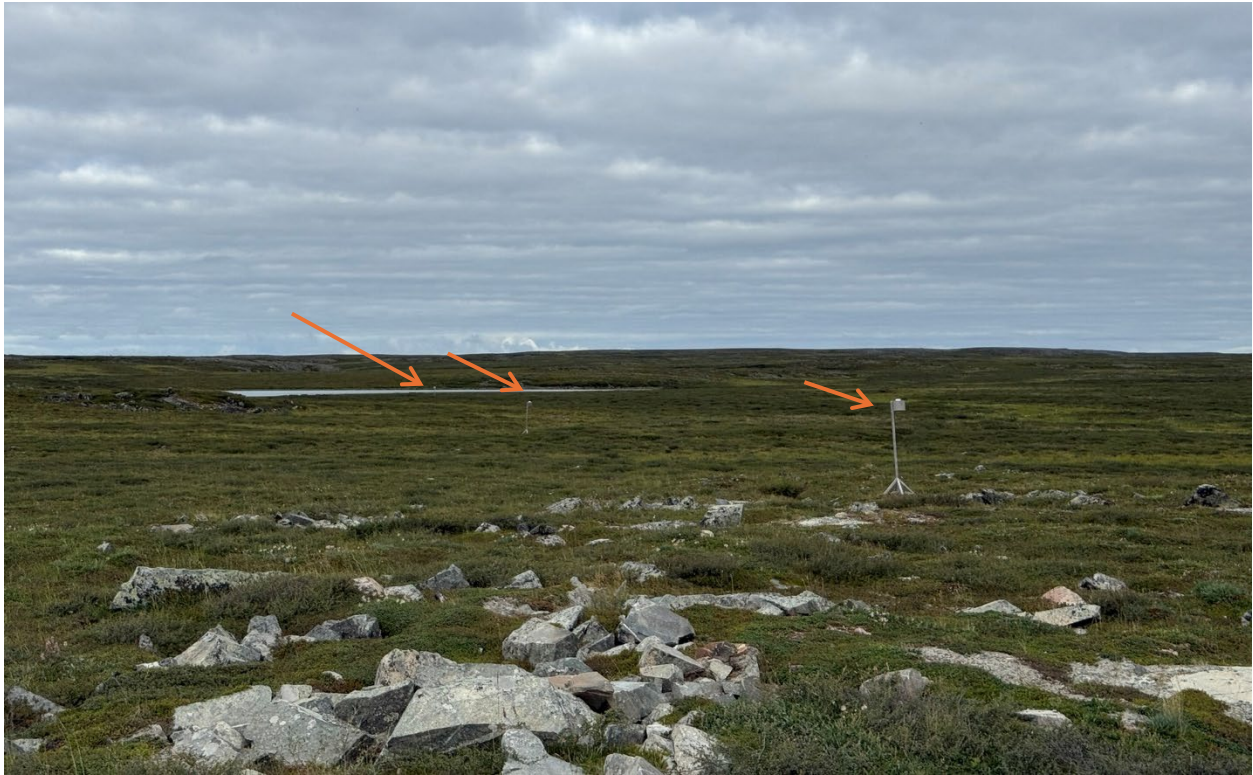
Photo 18: Dust monitoring transects at KM 18, with canisters positioned at set distances
