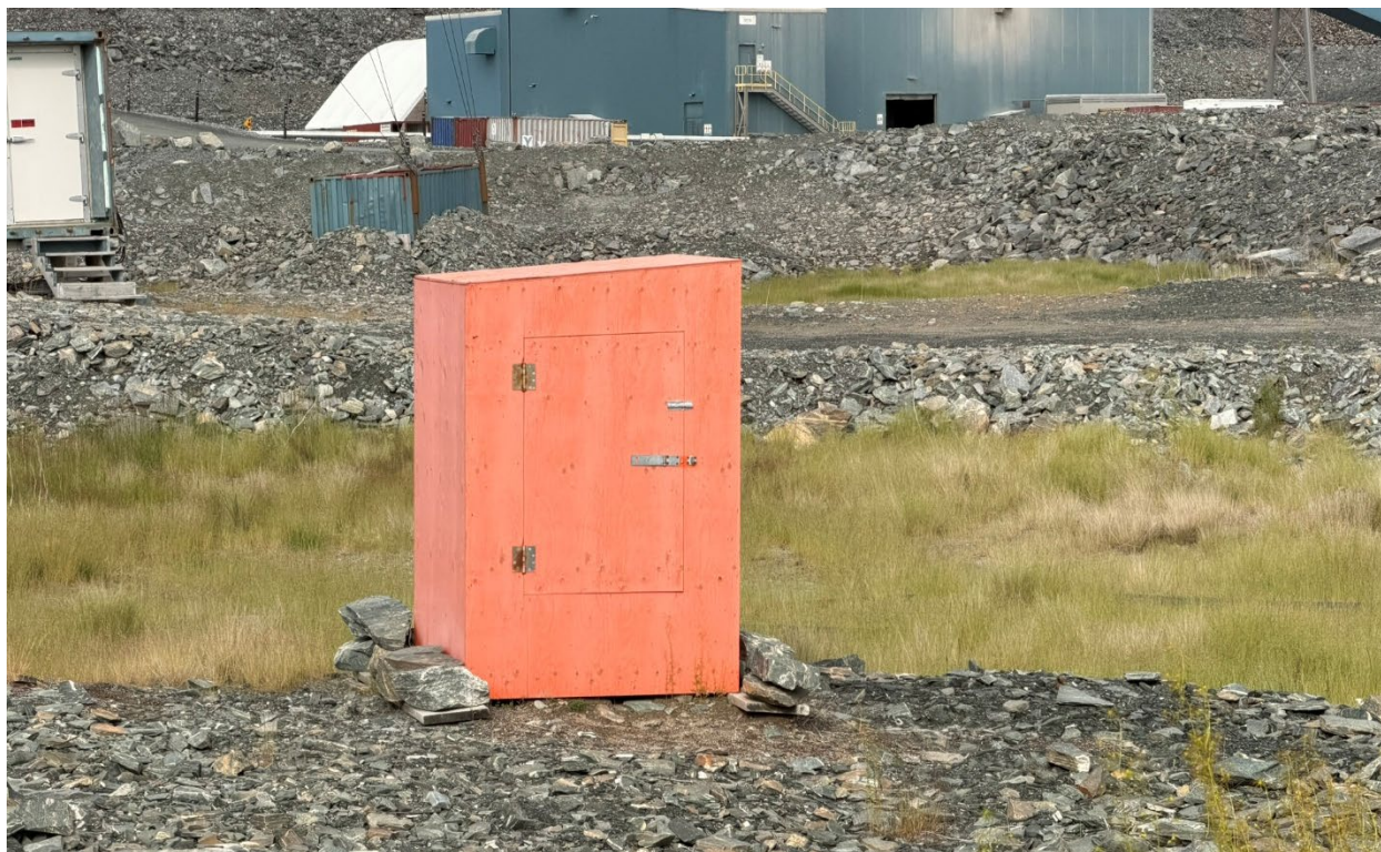
Photo 50: Surface blast and vibration monitoring station, monitors peak particle velocity and overpressure from blasting at TIRI01
