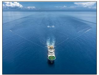
Figure 30: 3D Seismic Survey, Offshore Figure China (Source: Empyrean Energy, n.d., as cited in Nunami Stantec, 2018b)
